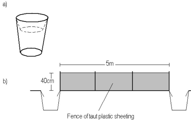
**Figure 1: a) The bucket design with a plastic basin inserted to stop caught animals escaping. b) A lateral profile of the pitfall design, showing the fence between two sunken buckets.**
