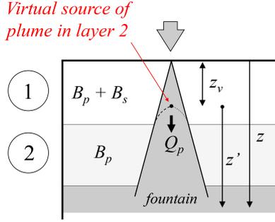
FIGURE 13. Virtual source of the particle-laden plume which descends through layer 2.
