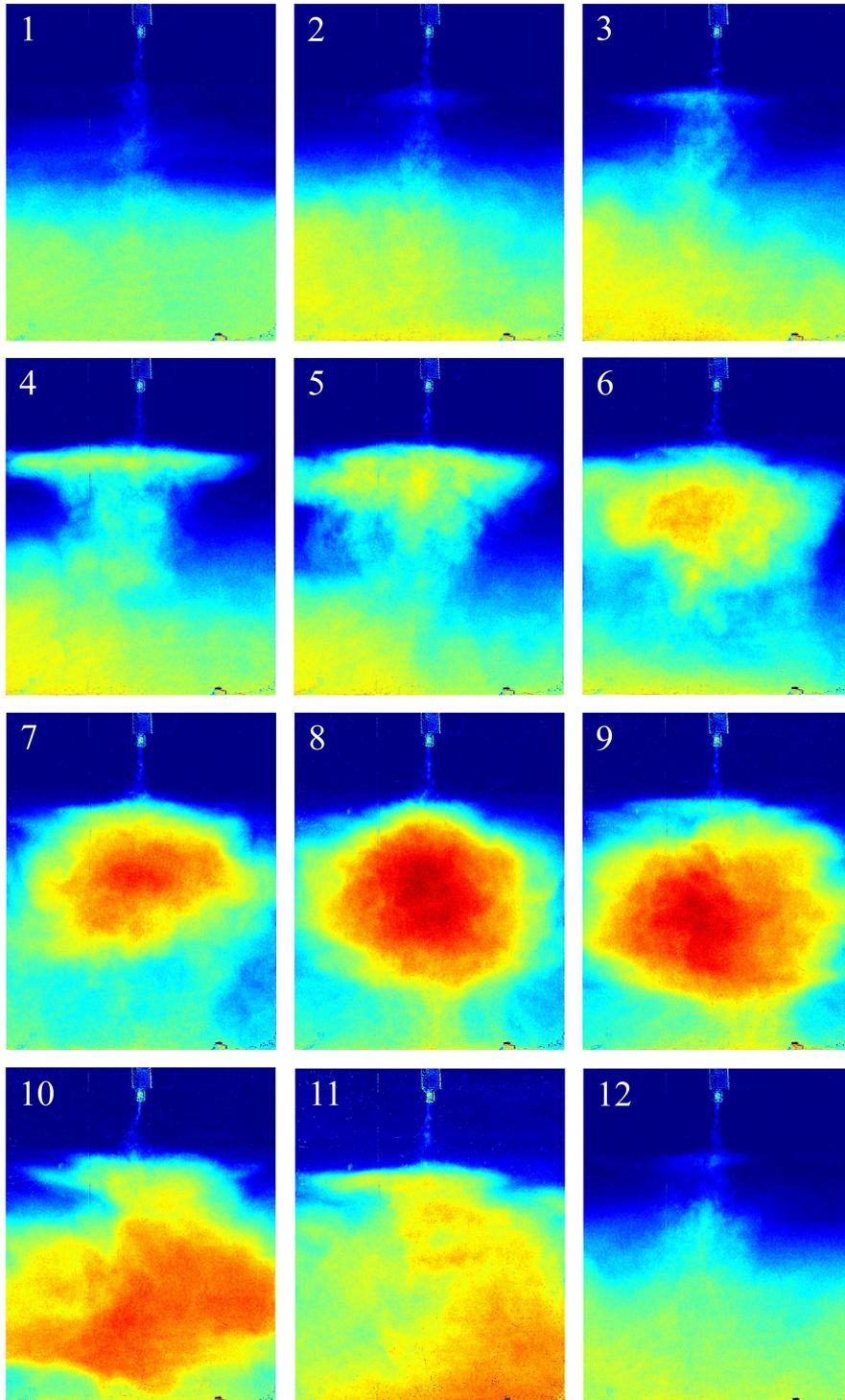
FIGURE 18. Large-scale instability observed during experiment h. Image 1 was captured 670 seconds after particles were added to the plume fluid at the beginning of the experiment. Images 2-12 were captured at the following times (relative to image 1): 220, 296, 352, 414, 490, 558, 652, 738, 862, 1212 and 1544 seconds.
