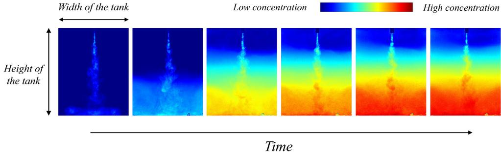
FIGURE 3. Transient concentration of particles in suspension in the tank during experiment b (cf. table 1). A series of images illustrate the concentration distribution in the tank at the following times after the beginning of the experiment: 30 seconds and 5, 28, 43, 70 and 86 minutes.
