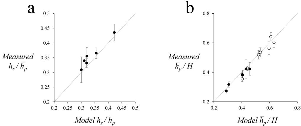
FIGURE 14. Comparison of experimental results with model predictions: a) distance between the plume source and the interface between layer 1 and layer 2,  $h_s$ ; b) distance between the plume source and the level at which particles with a mean settling speed  $\bar{v}_s$  are suspended in the ambient fluid,  $\bar{h}_p$ .
