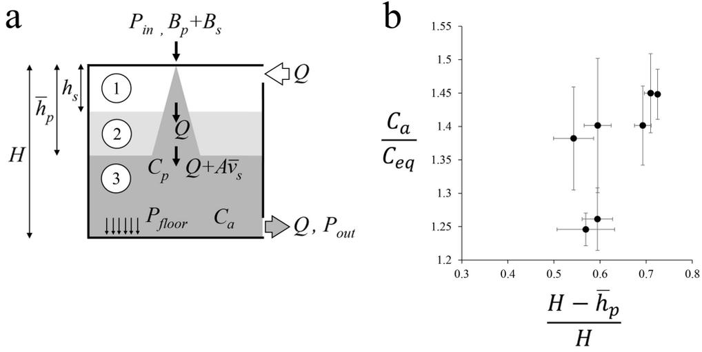
FIGURE 12. a) Cartoon showing the conditions used in the modelling (section 4); b) The measured concentration of particles at the base of the tank,  $C_a$ , is compared with the expected concentration  $C_{eq}$  given by equation 2.16.
