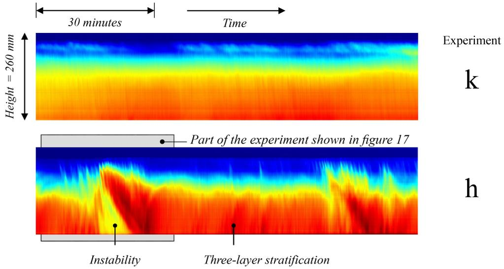
FIGURE 16. Transient horizontally-averaged mean concentration of particles in the tank in experiments k and h (cf. table 2). In experiment k, a steady three-layer stratification is observed (cf. section 4). In experiment h, we observe intermittent instabilities.
