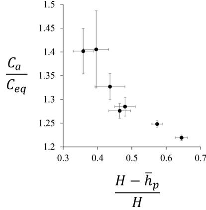
FIGURE 7. The measured concentration of particles at the base of the tank,  $C_a$ , is compared with the concentration  $C_{eq}$  given by equation 2.16. We observe that in our experiments  $C_a$  is consistently larger than  $C_{eq}$ .
