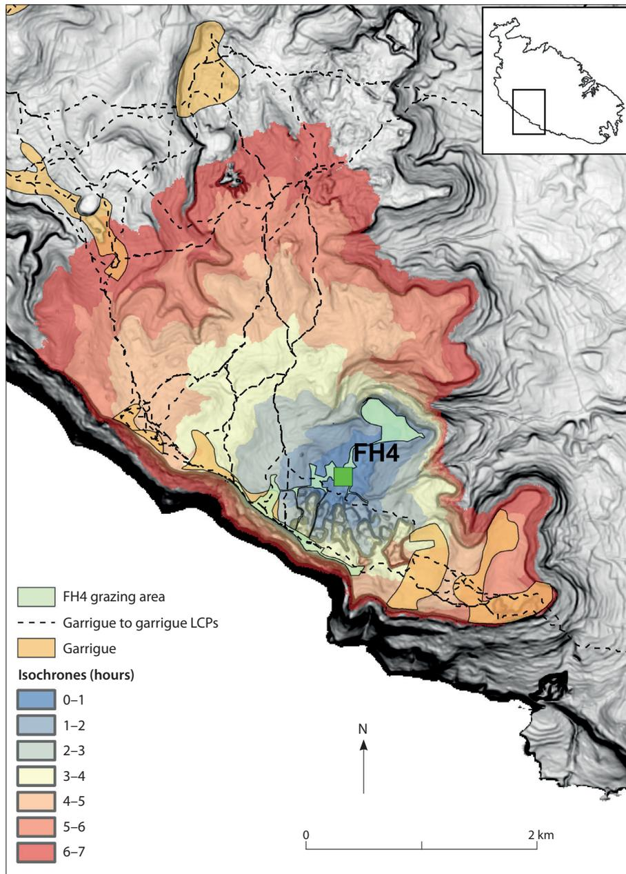
**Figure 9.11.** Isochrones around farmhouse 4 representing the space that can be covered at 1-hour intervals considering animal walking speed (grazing while walking; averaging 1.5 km/h on a favourable slope) (G. Alberti).
