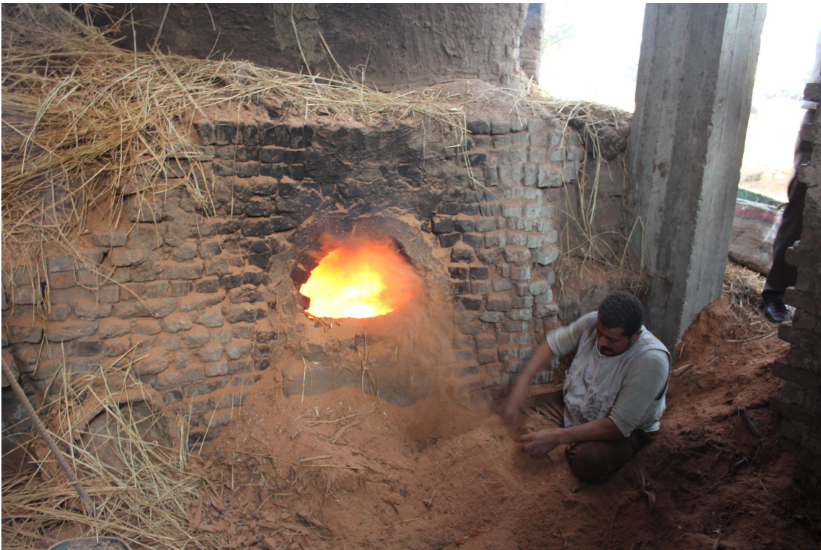
Figure 6.4. Adding sawdust to an initial firing at Rahmaneyah (photo Heike Möller).
