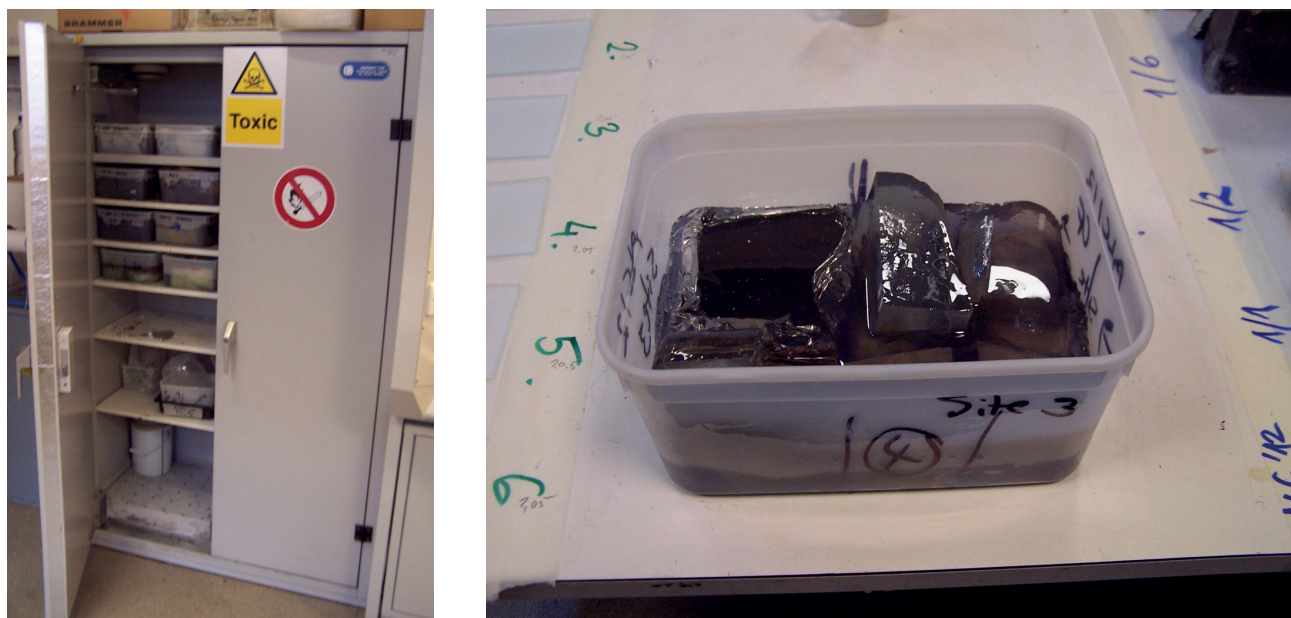
Figure 7.4. Curing of impregnated blocks: left, cabinet for curing impregnated blocks; right, impregnated block ready for sawing. Images: Tonko Rajkovaca.
