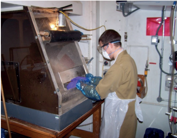
Figure 7.5. Sawing: left, a. the electric saw used to cut impregnated blocks; right, slides of 4–5mm thickness cut, the top side is marked with a notch. Images: Tonko Rajkovaca.
