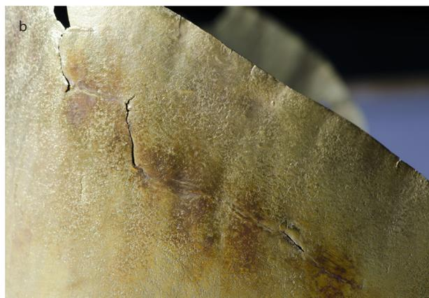
**Figure 6.41.** Stress-induced corrosion of (a) a fracture in an Iron Age earring and (b) a crack in an Early Bronze Age diadem (Au 835 and Au 133, National Museum of Archaeology, Portugal).
