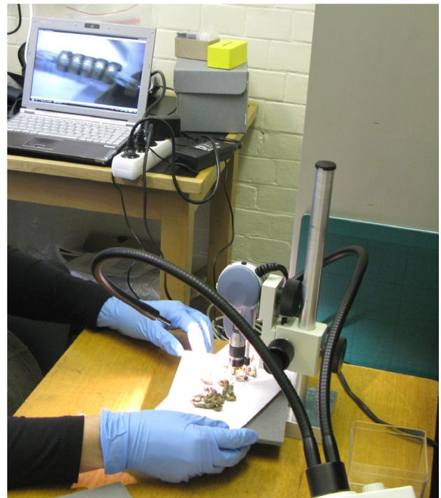
**Figure 6.1.** Working at the Petrie Museum with the compact high-resolution Flexia video microscope from Optilia with a colour 5.0 MP CMOS image sensor ( $2592 \times 1944$ ), a zoom reaching  $\times 100$ , a built-in LED illumination and a Bersoft image measurement software.
