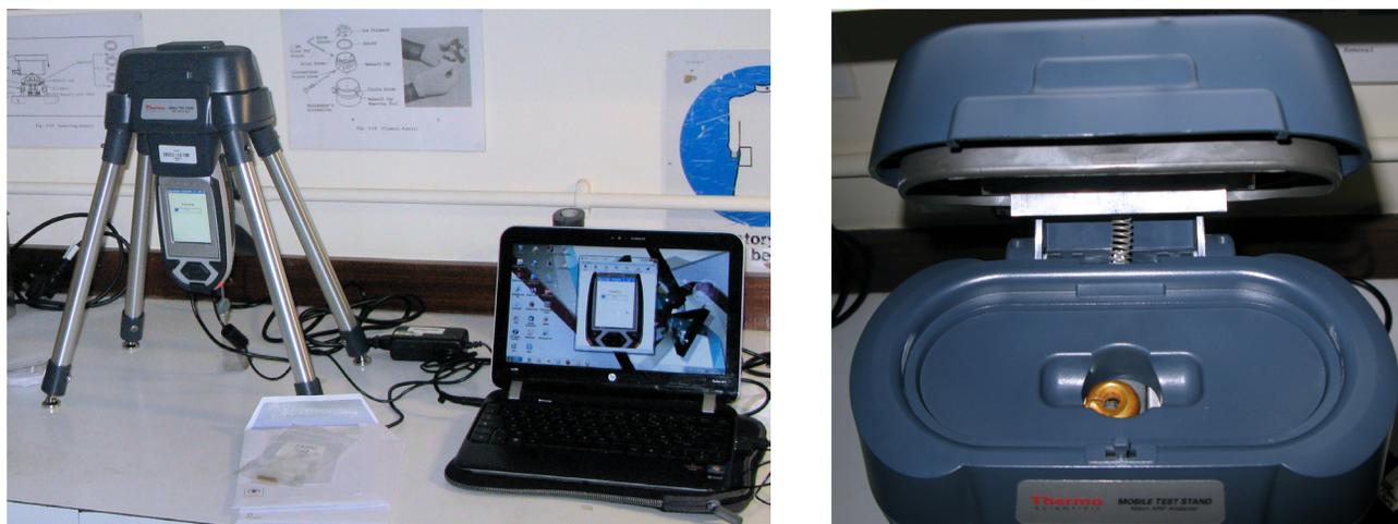
**Figure 6.16.** Analysis of penannular earring 6146b from Riqqa, in the collection of the Manchester Museum, using the handheld XRF equipment of the University of Liverpool.
