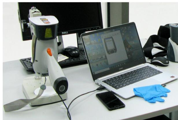
**Figure 6.15.** The handheld XRF equipment of the C2RMF with its lightweight stand.
