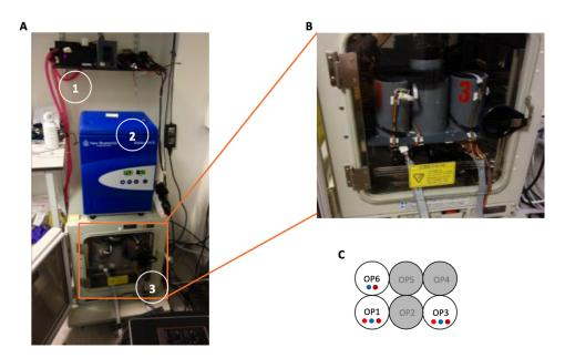
Fig. 3.15 A) The *OptoFarm* includes a water-cooling system (1) for the electronics, a small incubator (2) and a medium-sized incubator (3) containing 'optoPODs' (B), with LED ights installed at the bottom. C) Schematic of the optoPOD setup inside the incubator. Only three optoPODs are operational (coloured) with the shown lights (as dots), ie blue, red and infrared.
