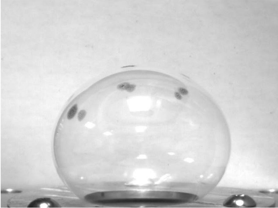
**Figure 3.14:** Photograph of an inflated rubber sheet during bulge test. Reprinted with permission from Cambridge Polymer Group.
