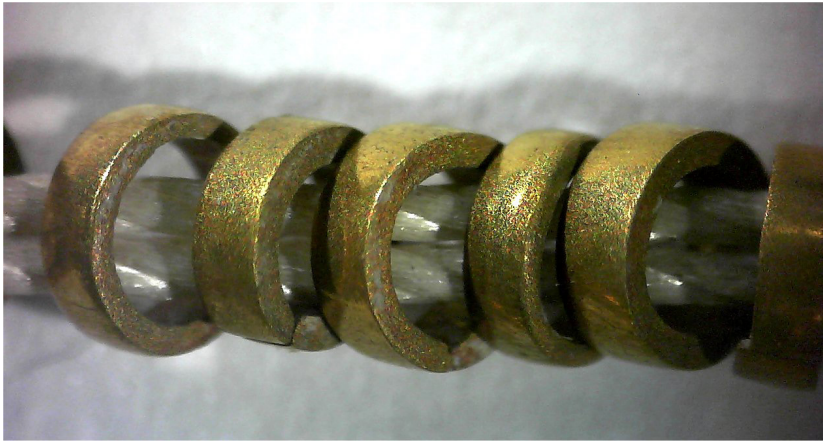
Figure 7.29. The quite regular ring beads of string UC20649 and one of their visible PGE inclusions.
