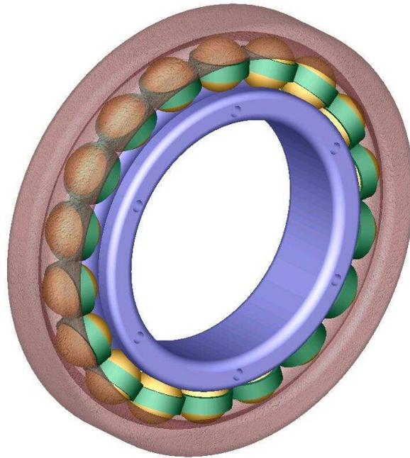
Figure 6.1: Schematic representation of a ball-bearing, formed from an inner ring blue, an outer ring purple and the balls yellow which are kept aligned by a cage green.
