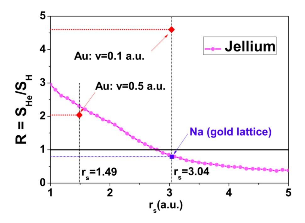
Static impurity screening: a change in electronic distribution in adiabatic states without the impurity
