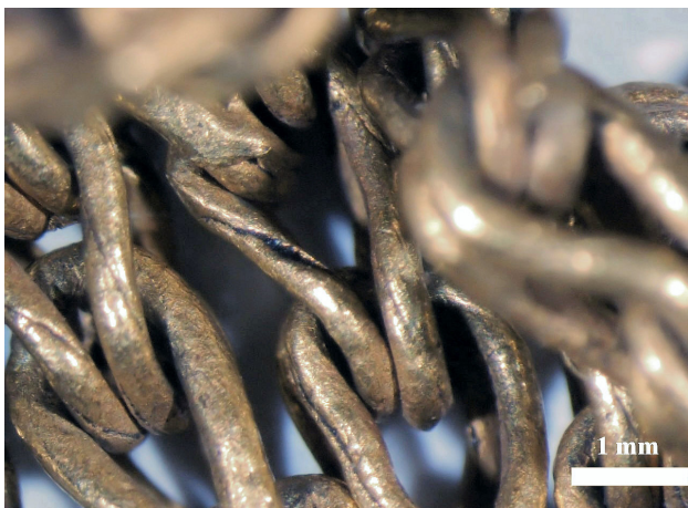
Figure 10.81. Details of the loop-in-loop chain E2990A showing the longitudinal seams typical of the use of strip twisting and the thick soldered joint of the links.
