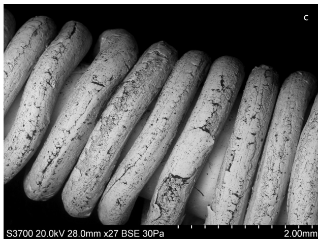
Figure 10.38. (a) SEM-BSE image of the bezel and end shanks of finger-ring EA 2923, (b) a detail under the stereomicroscope of the coiled single wire entering into the bezel through the gold cup, and (c) SEM-BSE image of the hammered wire showing longitudinal creases smeared over.
