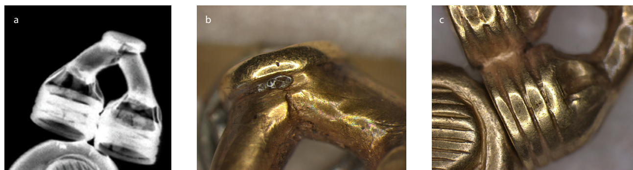
Figure 10.71. The lotus terminal of string EA14696: (a) X-radiographic image revealing the different soldered components, including the individual wire loops (BM X-ray plate 6900/1, 10 mA, 100 kV, 2 min, lead screen, Structurix film D4) and (b,c) details of the lotus stems under the stereomicroscope showing the soldered joins of components.
