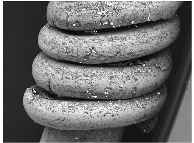
Figure 10.43. Creases from hammering and rolling visible at the surface of the coiled shank of finger-ring AF2462.
