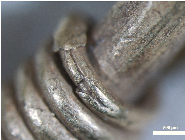
Figure 10.43. Creases from hammering and rolling visible at the surface of the coiled shank of finger-ring AF2462.
