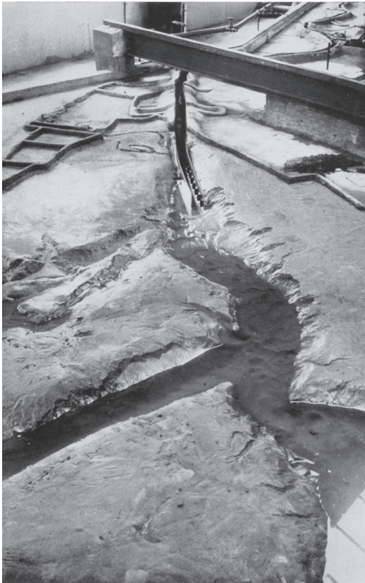
Figure 8.4. Ouse Tidal Model: left, in demonstration 'flow' and, lower right, under construction (from Doran 1941); upper right, sketch rendering of the model's plunger system (Allen 1947, fig. 97). Operating the model may well have taken its toll. Apart from the fact that the shed's roof and walls were apparently of asbestos, a Pathe film of 1950 (Fens Model) recording its operation actually has men pouring mercury down its channels. This must have been to enhance the model's demonstration purposes, as the operation of a 'mercury-flow Ouse' would surely not equate with that of the river's waters. Images: Andrew Hall.
