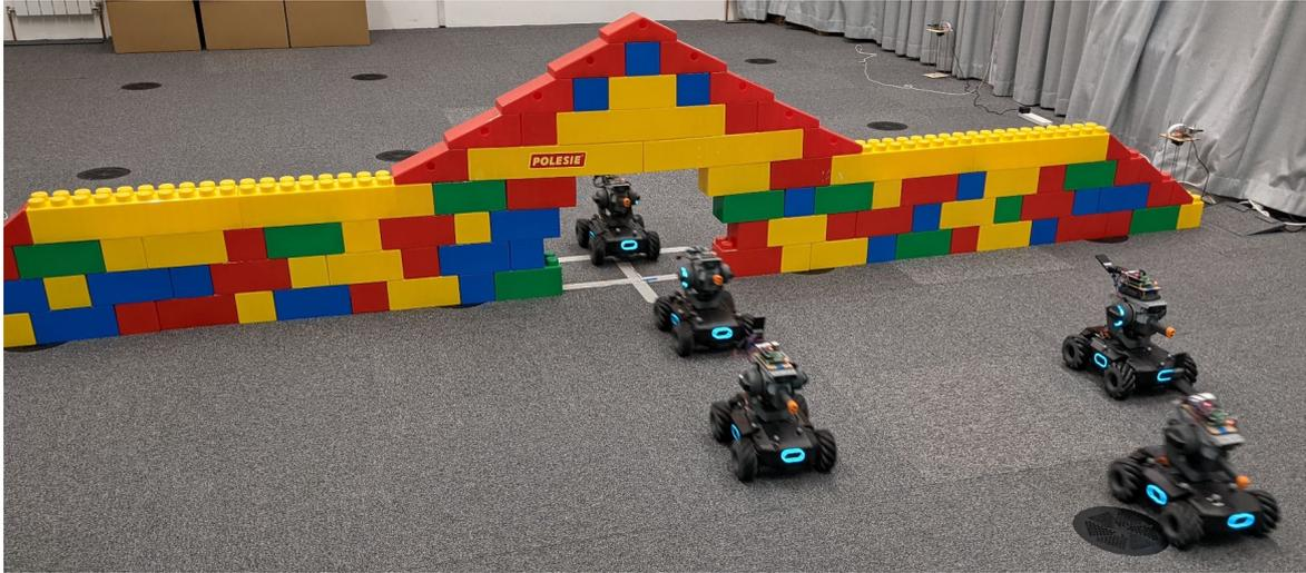
Fig. 4.4 We deploy a set of five DJI RoboMaster robots in a real-world setup using GNNs and Adhoc communication. The robots navigate through a narrow passageway to reconfigure on the other side, as quickly as possible.
