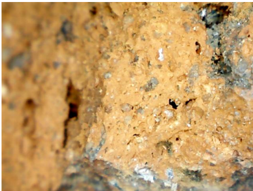
Figure 37: Fabric T12 fresh break 6mm across
