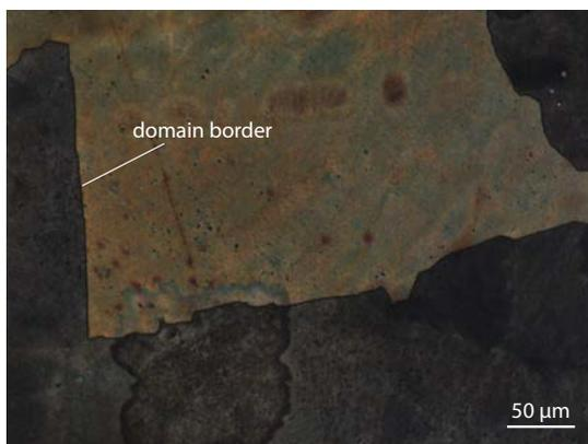
Figure 3.5: Domain morphology of gyroids obtained by drying-annealing. The image was obtained by optical microscopy under linear polarized light after metal replication. As discussed in the next chapter, the metal gyroids show a strong linear dichroism that enables the inspection of the domain size by optical microscopy.
