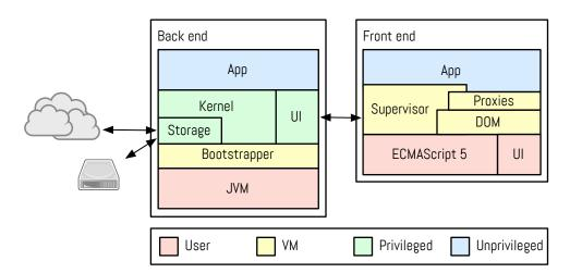
Figure 5.3: Applications are split into front-end and back-end components.
