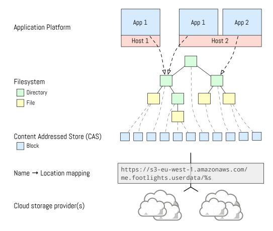
Figure 4.1: Footlights and its static storage layers.
