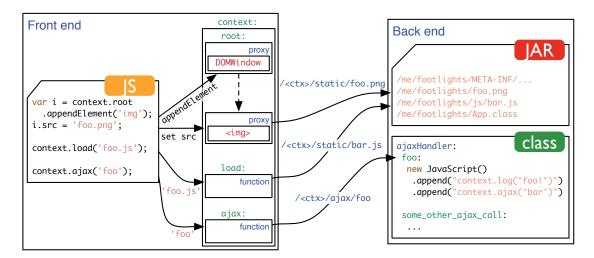
Figure 5.6: Communication over a multiplexed HTTP channel.
