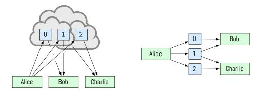
Figure 4.9: Block upload/download is equivalent to multicast messaging.
