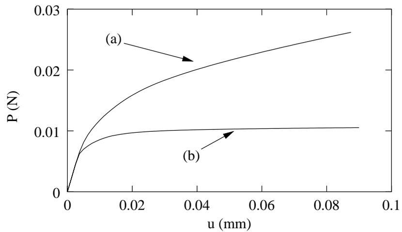
Figure 8: Load–displacement response for the three-dimensional punch test with (a) linear tetrahedra and (b) enhanced tetrahedra.
