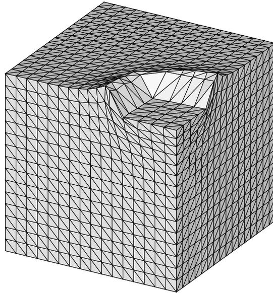
Figure 7: Deformed three-dimensional mesh for the punch simulation. Using symmetry, only one quarter of the block is modelled.
