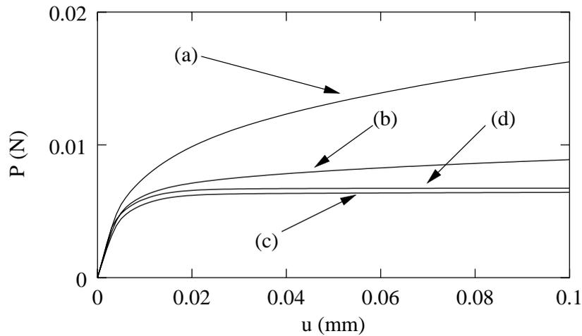
Figure 5: Load–displacement response for the axisymmetric punch test with (a) diagonal linear triangles, (b) crossed linear triangles, (c) diagonal quadratic triangles and (d) diagonal linear triangles with enhancement.
