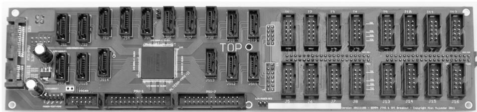
Figure 5.4: Parallel programming and status monitoring board
