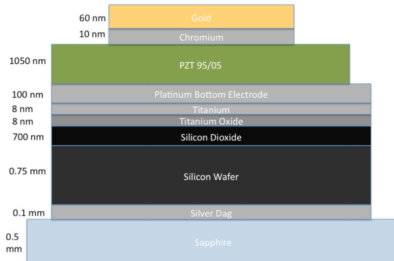
**Figure 3-1. Cross section of PZT 95/05 sample mounted on sapphire disc.**
