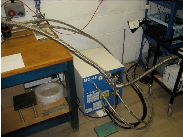
**Figure 3-9. Compressor and vacuum pump.**
