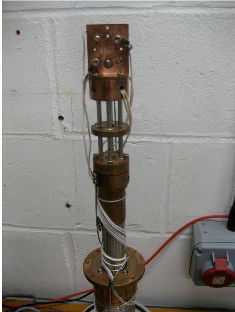
**Figure 3-11. Cold stages and sample stage.**
