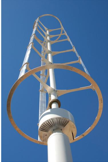
Figure 3.9: Photo of the high aspect ratio WindSpire turbine (image from the WindSpire website)
