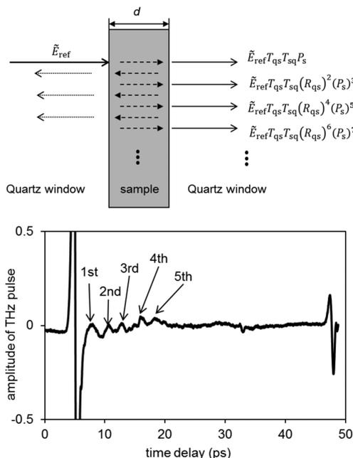
**Figure 1.** Single-slab model of terahertz radiation propagating through the liquid cell (top). Identification of echo pulses originating from the multiple reflections within the sample layer (bottom).
