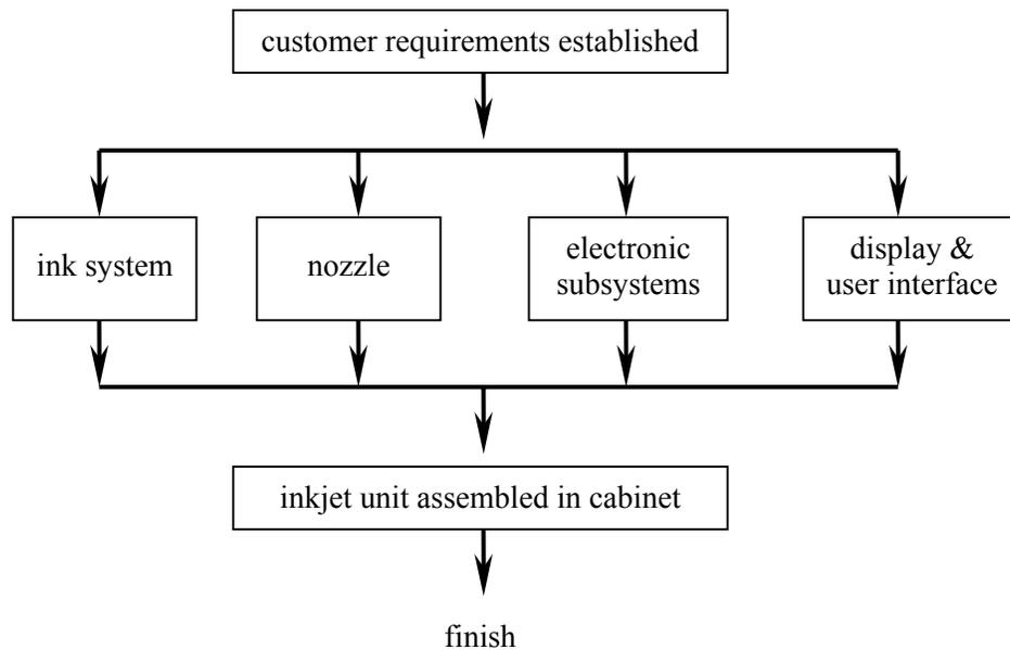
**Figure 6.3: Manufacturing Procedure for Domino's Inkjet Printers**
