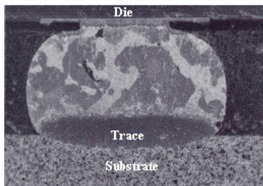
**Figure 5.6: C4 Connection between Packaging and Die**<sup>31</sup>
