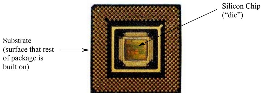
**Figure 5.1: A Silicon Chip Mounted in a Typical Packaging Unit**<sup>26</sup>
