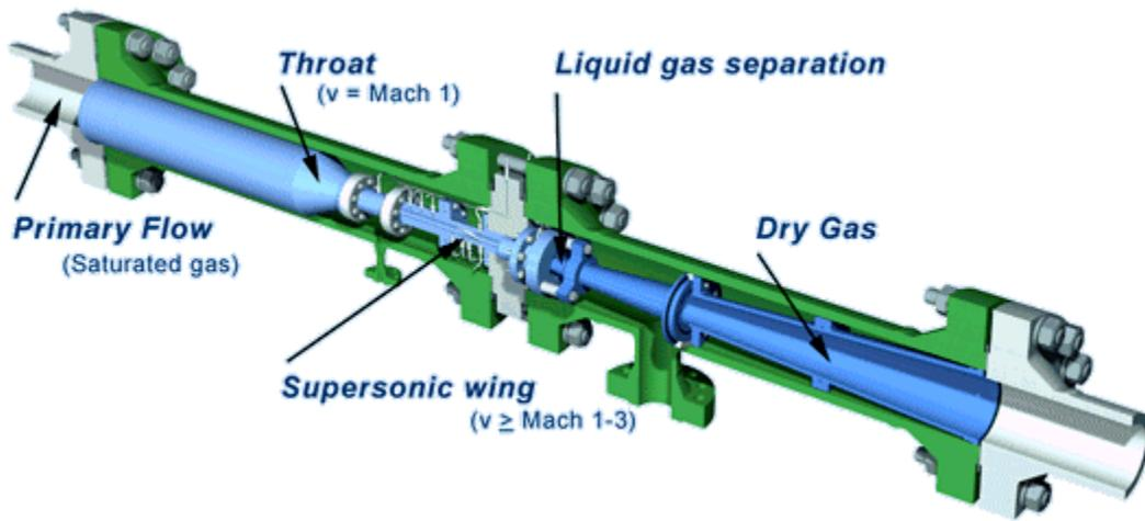
**Figure 7.3: The Twister Cyclone Separator—Cross Section**<sup>51</sup>
