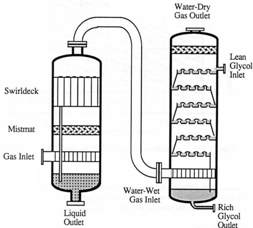
Figure 7.1: A Typical Separator and TEG Contactor
