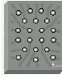
**Figure 5.5: Control Collapse Chip Connect (C4) Ball Array**<sup>30</sup>
