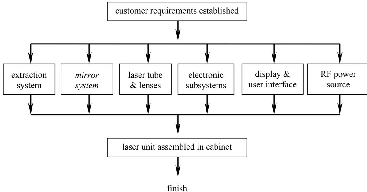
**Figure 6.6: Manufacturing Procedure for Domino's Laser Printers**
