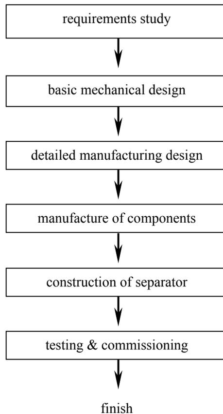
**Figure 7.5: Manufacturing Procedure for Twister Separators**
