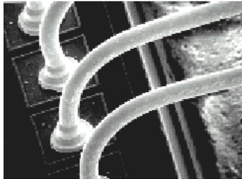
**Figure 5.4: Scanning Electron Micrograph of Wire Bond Between Die and Packaging**<sup>28</sup>
