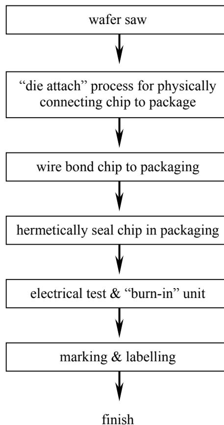
**Figure 5.3: Manufacturing Procedure for Ceramic/Wire Bonding Packaging**
