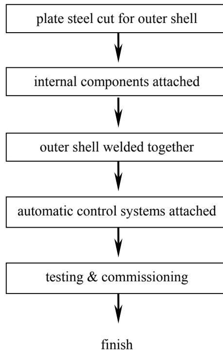
**Figure 7.2: Manufacturing Procedure for Separators, Contactors, and Reboilers**
