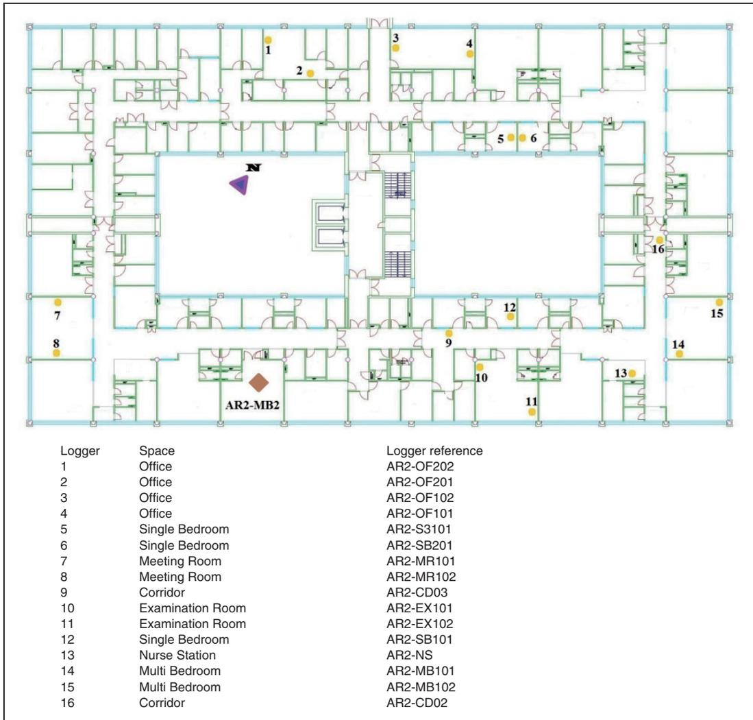
**Figure 2.** Monitored spaces and logger locations in Rosie level 2. AR2-MB2 was considered for predicted performance analysis.
