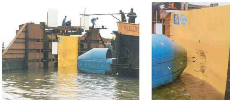
**Figure 2.21:** Photographs of full-scale collision tests performed on the Y-frame double hull structure. Adapted from Konter et al. (2004) and Wevers and Vredeveldt (1999).
