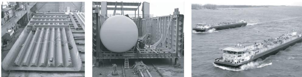
**Figure 2.22:** Construction of inland waterway tankers with a Y-frame single hull structure. Adapted from Graaf et al. (2004) and Vredeveldt and Roeters (2004).
