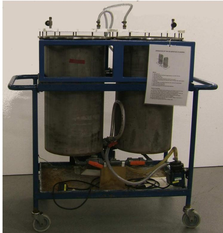
**Figure 2.8:** Dissolved air is removed from solution by depressurisation in these stainless steel cylinders.
