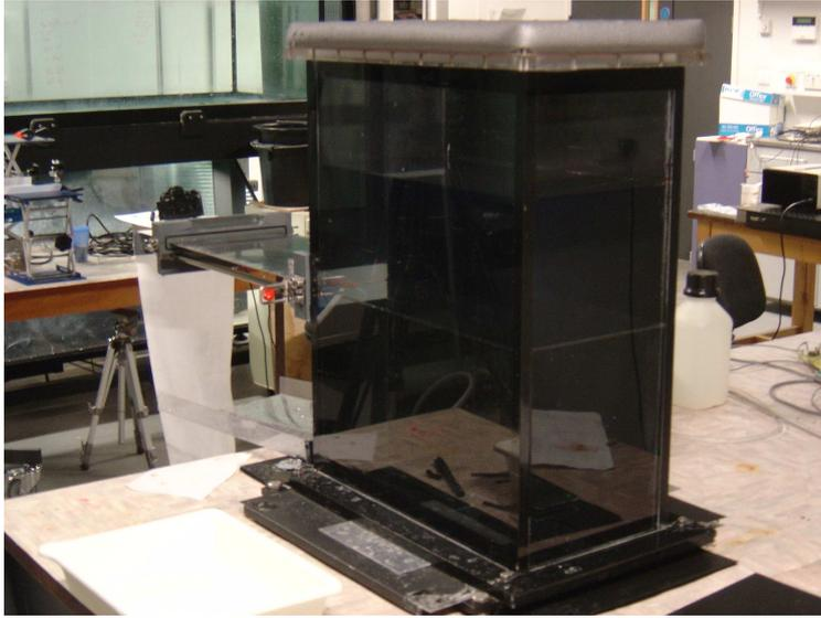
**Figure 2.1:** Low aspect-ratio Rayleigh-Taylor box, showing its barrier fully withdrawn.
