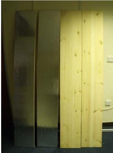
Figure 5: 300mm louvers made from timber. One face of the louvers was covered with reflective aluminium tapes.
