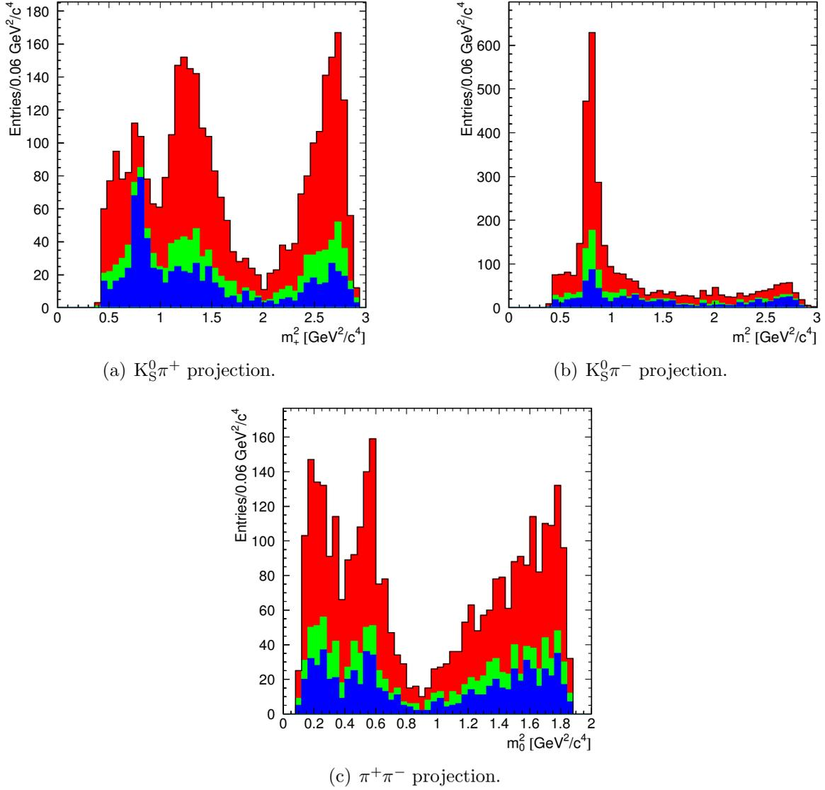
**Figure 6.10:** The Dalitz projections for the Belle Isobar model fit scenario including the acceptance, DK-random background at  $B_{DK\text{-rand}}/S = 0.35$  (dark blue),  $D\pi$ , DK-signal and  $D^*$  backgrounds at  $B_{D\pi,DK\text{-random},D^*}/S = 0.21$  (green). The data corresponds to  $2\text{ fb}^{-1}$  and the signal is shown in red.
