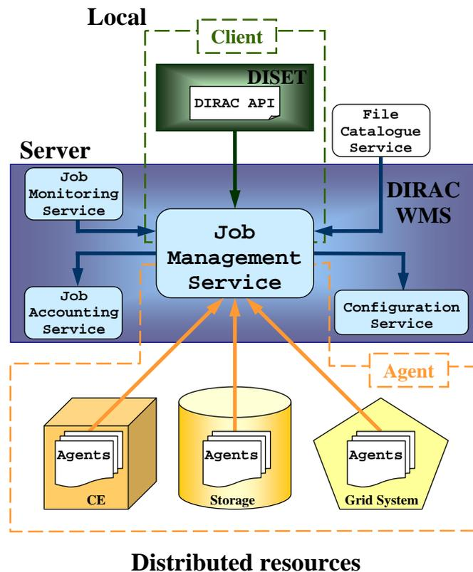
**Figure 3.2:** General overview of the DIRAC architecture. Areas of the Client (green) and Agents (orange) are highlighted in dotted lines. Some of the main DIRAC services are also shown in blue boxes. The arrows indicate the communication path between the components.
