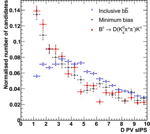
**Figure 4.8:** The LL and DD combined D PV sIPS distribution for the inclusive  $b\bar{b}$ , minimum bias and signal samples passing all preselection cuts. A unitary normalisation is applied to all three distributions.
