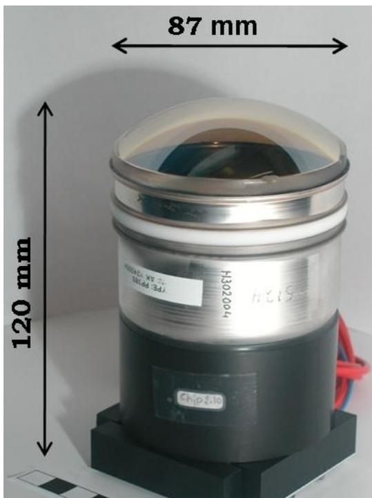
**Figure 2.23:** A completed HPD module.
