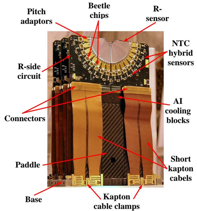
**Figure 2.16:** A fully assembled and mounted VELO module.
