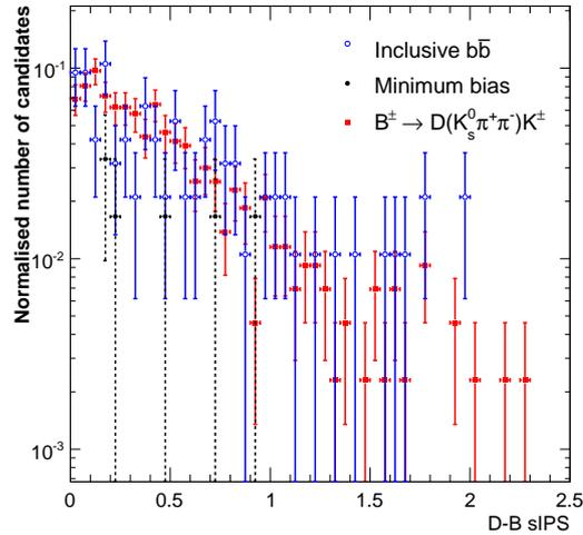
**Figure 4.9:** The LL and DD combined D-B sIPS distribution for the inclusive  $b\bar{b}$ , minimum bias and signal samples passing all preselection cuts. A unitary normalisation is applied to all three distributions.
