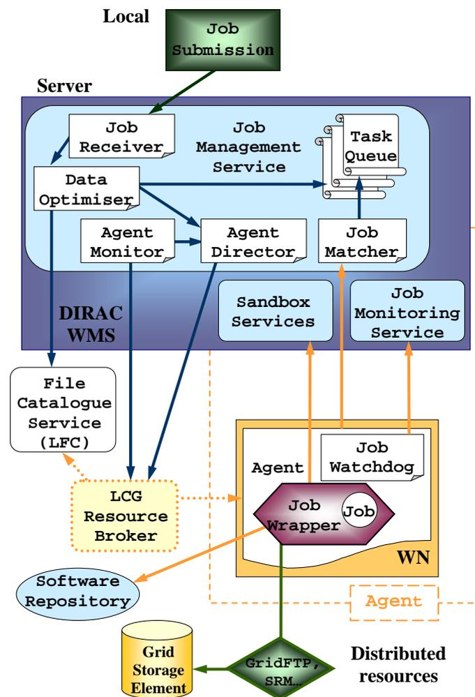
**Figure 3.6:** Overview of CPU resource Agent setup showing the communication between components on the WN with the WMS, data storage via a secure protocol (e.g. GridFTP) and to the LCG RB in the case of Pilot Agents.
