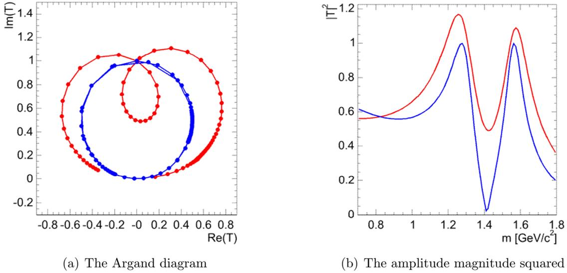
**Figure 6.3:** The Argand and amplitude plots for the BW (red) and K-matrix (blue) formalisms with two strongly overlapping resonances. It can be seen in (a) in the BW parametrisation violates the unitarity condition, while the K-matrix parametrisation respects it. In terms of the resulting amplitude magnitudes, the K-matrix formalism produces a line shape containing a much stronger destructive interference between the two resonances as shown in (b) [197].
