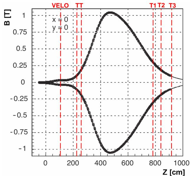
**Figure 2.19:** The measured LHCb dipole magnetic field along the  $z$  axis in both polarities [75]. The points show the measurements taken from the VELO, dipole magnet, tracking stations and also inside the magnetic shielding for the RICH system. The solid lines are the result of the model calculations.
