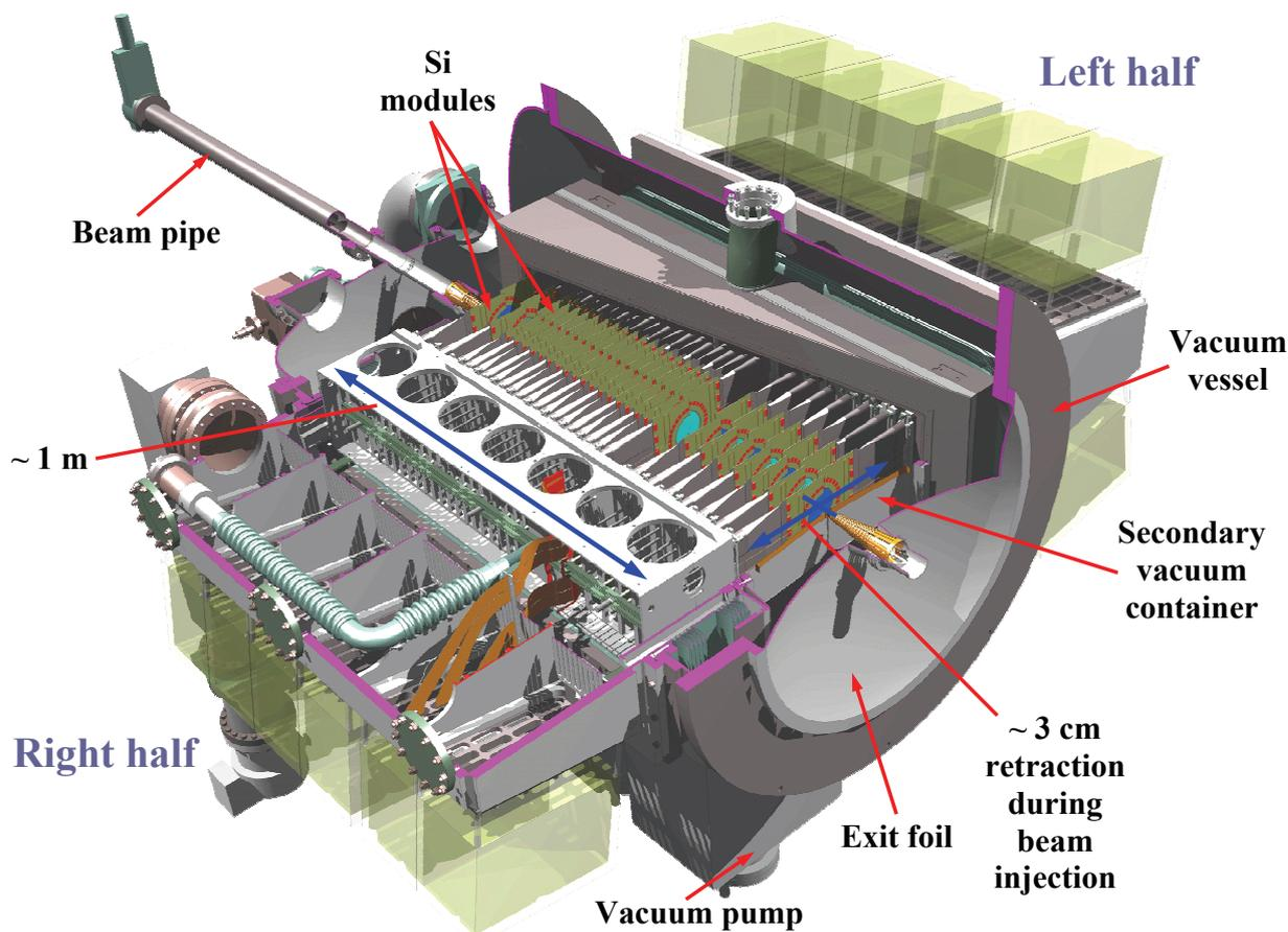
**Figure 2.11:** A cut away schematic of the VELO detector showing the two retractable silicon module halves and the vacuum enclosure system. The VELO is shown with the dipole-magnet end facing the bottom right-hand of the diagram.
