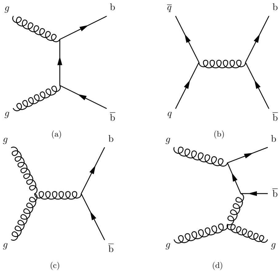
**Figure 2.5:** Feynman diagrams of dominant  $b\bar{b}$  pair production mechanisms at the LHC. (a) shows the gluon-gluon fusion, (b) shows the quark-antiquark annihilation, (c) shows the gluon splitting and (d) shows flavour excitation.
