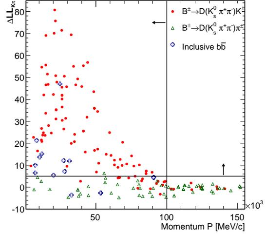
**Figure 4.14:** DC06 LL event distribution for momentum versus  $\Delta LL_{K\pi}$ . The vertical and horizontal lines indicate the momentum and  $\Delta LL_{K\pi}$  cuts respectively.
