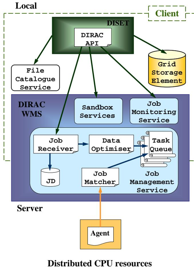
**Figure 3.3:** Outline of the DIRAC Client modules, the functionality and relations between the modules and Services is given in the text.
