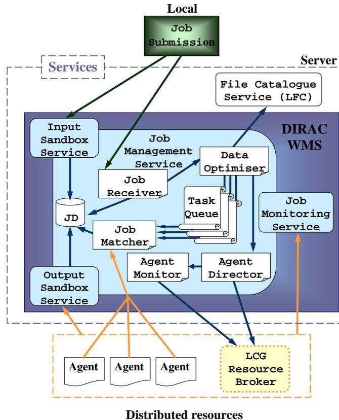
**Figure 3.5:** Overview of the DIRAC WMS, with its main components and Services. The arrows show the information transfer between the components, linking the Services with the distributed resources. The functionality of the components is given in the text.
