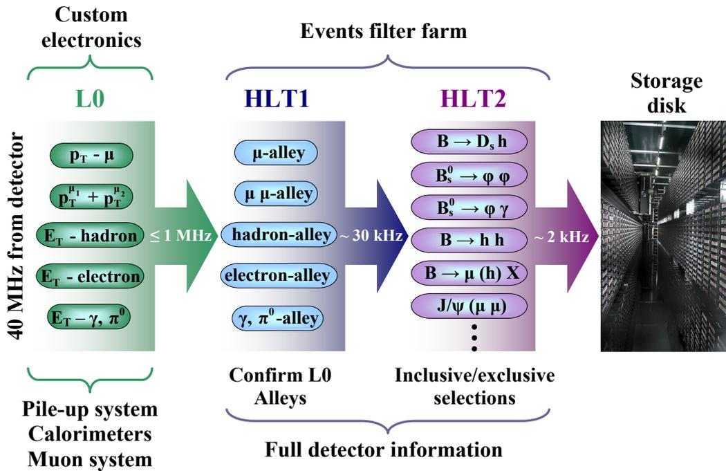
Figure 2.35: The overview of the LHCb trigger system.
