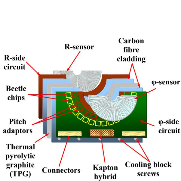
**Figure 2.15:** A 3D blow-out of the VELO hybrid silicon sensor construction.
