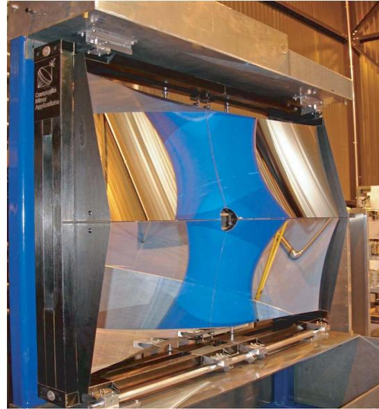
**Figure 2.26:** The completed RICH1 spherical mirrors.
