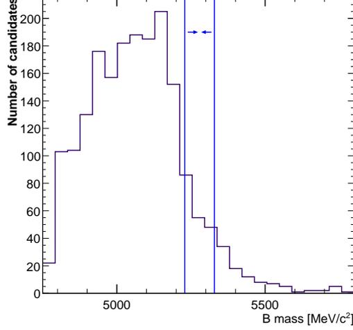
**Figure 5.12:** Reconstructed B mass distribution from the DX sample in the  $\pm 500 \text{ MeV}/c^2$  B mass window with a relaxed particle identification on the bachelor kaon. The tight  $\pm 50 \text{ MeV}/c^2$  mass window is shown. No trigger is applied.
