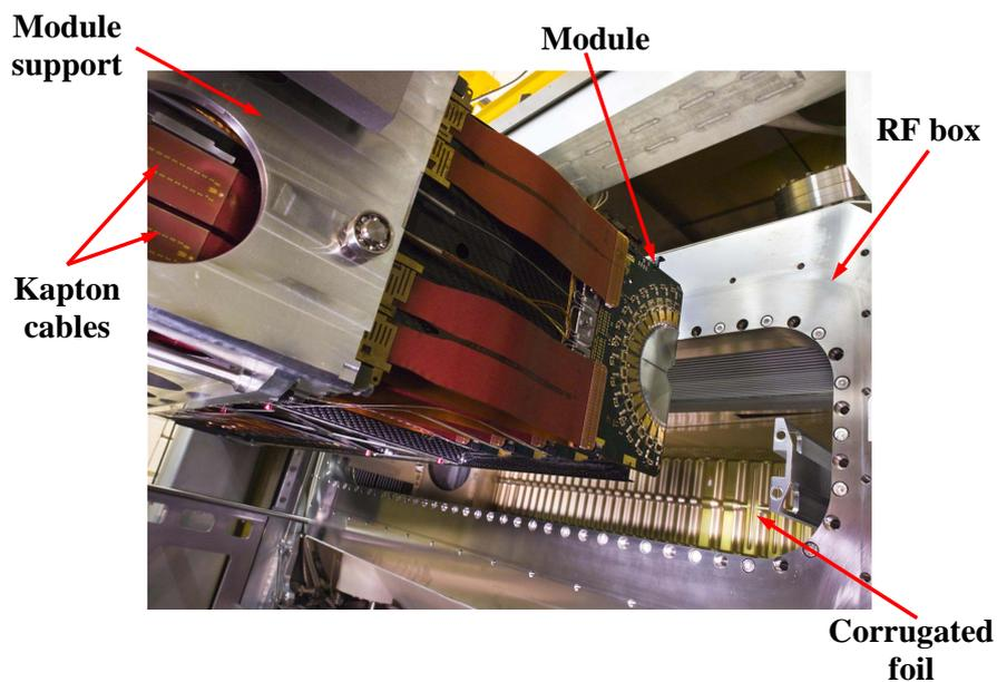
**Figure 2.17:** Photo of one half of the fully mounted and installed VELO sensors, including the RF vacuum box and the movable module support.
