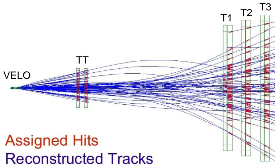
**Figure 2.20:** Reconstructed tracks from a typical LHCb event, showing simulated hits in the TT and the three trigger stations, T1-T3. The high track occupancy of the TT and the centre region of the tracking stations is seen.
