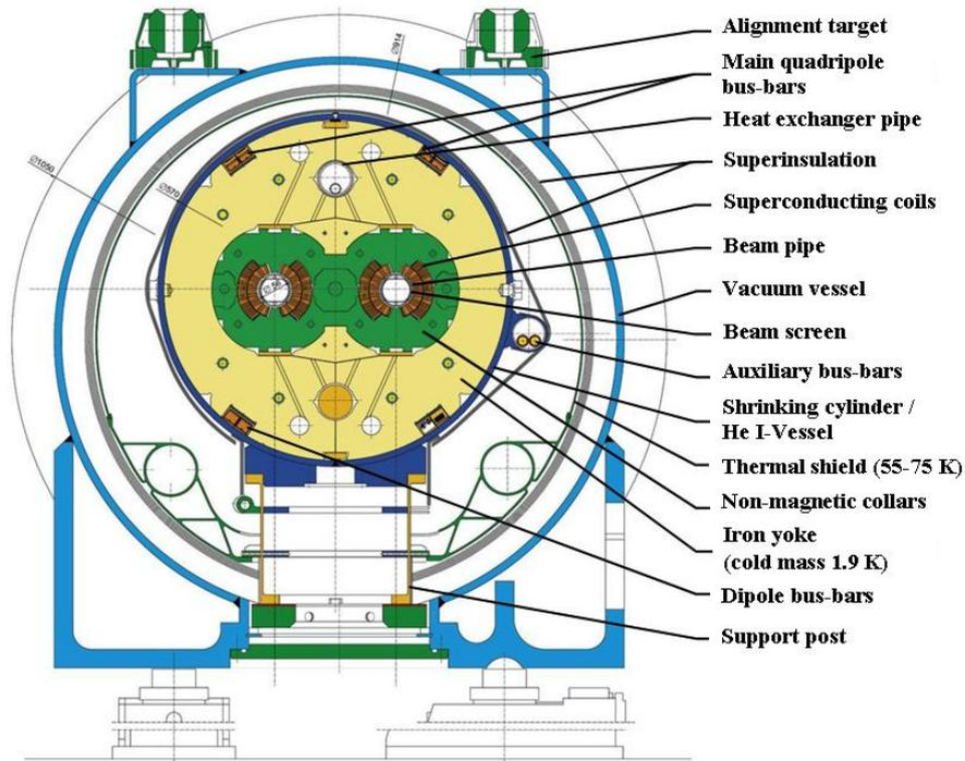
**Figure 2.4:** A LHC dipole magnet cross-section schematic [79].
