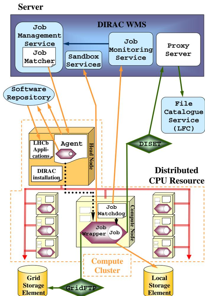
**Figure 3.8:** Compute Cluster compute element architecture overview with DIRAC Agent components shown. The arrows indicate the paths of communication between the components, with the dotted and double arrows showing the internal Compute Cluster communication paths, while the solid arrows indicate external communication. The functionality of the components are described in the text.
