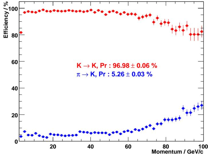
**Figure 2.30:** Particle identification of kaon and pion separation, where  $K \rightarrow K$  is the efficiency for identifying a kaon as a kaon, while  $\pi \rightarrow K$  is the efficiency for a pion to be mis-identified as a kaon [75].
