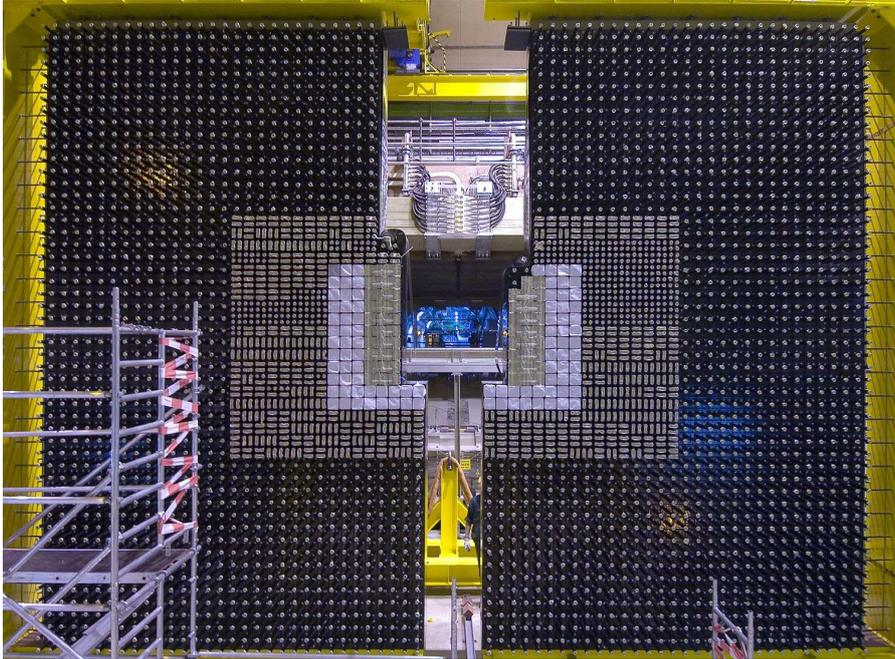
**Figure 2.32:** The near to completion ECAL as viewed facing upstream of the spectrometer. The two halves are shown with a few missing modules around and above the beam pipe window. The three sections of differing segmentation around the beam pipe window can be seen.
