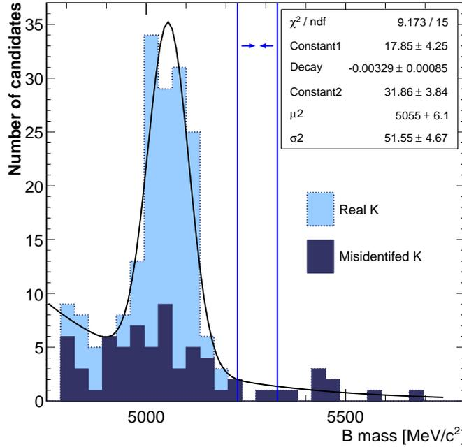
**Figure 5.14:** The reconstructed B mass distribution from  $B^\pm D^*$ ,  $B^\pm D^{*0}$ ,  $B_d^0 D^*$  and  $B_s^0 D^*$  samples in the wide  $\pm 500 \text{ MeV}/c^2$  mass window. The tight  $\pm 50 \text{ MeV}/c^2$  B mass window is indicated. No L0 trigger is applied. Contributions to the distribution from a real kaon and a misidentified kaon are also shown.
