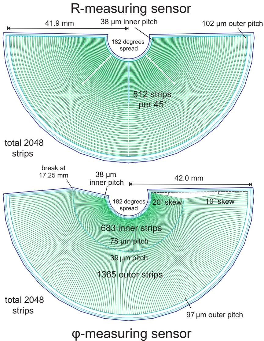
**Figure 2.14:** The R and  $\phi$  sensors.
