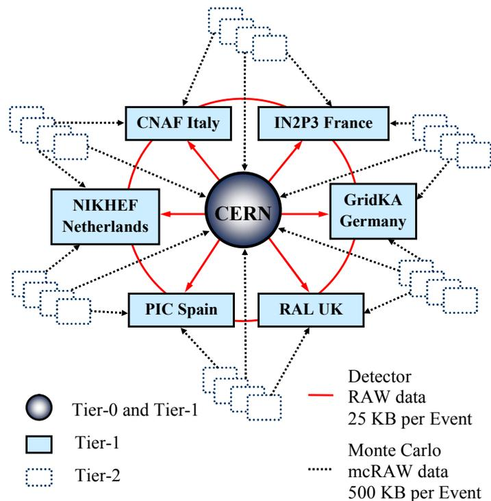
**Figure 3.1:** LHCb tier model and data transfer rates between the tiers. The arrows show the direction of data flow between sites.
