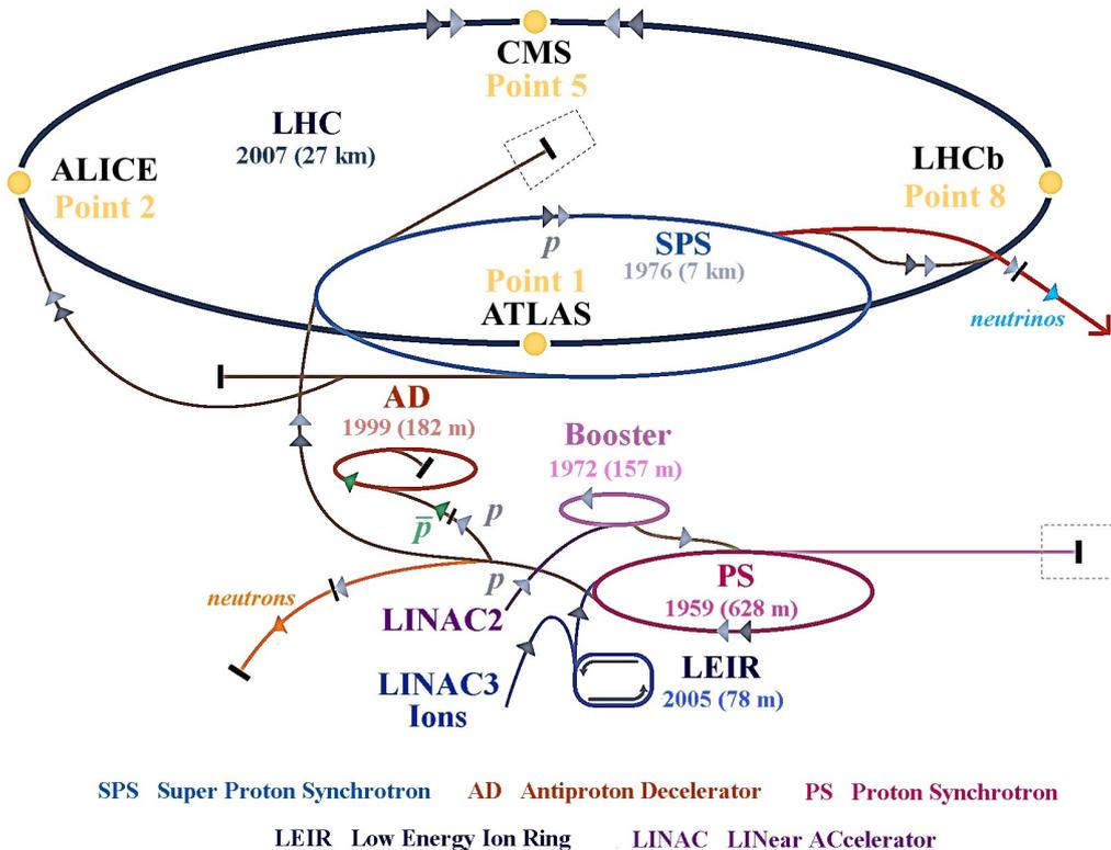
**Figure 2.2:** A schematic of the CERN accelerator complex.
