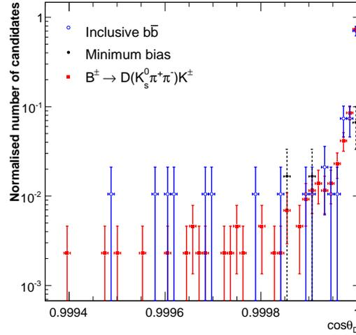
**Figure 4.10:** The LL and DD combined  $D \cos \theta_D$  distribution for the inclusive  $b\bar{b}$ , minimum bias and signal samples passing all preselection cuts; the preselection cuts tend to select background arising from  $B \rightarrow DX$  decays. A unitary normalisation is applied to all three distributions.
