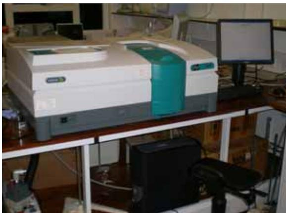
**Figure 3.11** Varian Cary 4000 UV/Vis spectrophotometer
