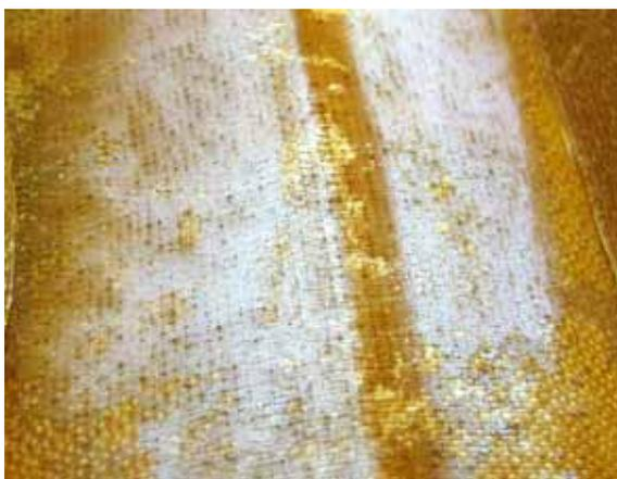
**Figure 5.7a** Photo of catalyst after double pass flow experiment with HIHO. The yellowish brown area indicates the adsorption of iron on the catalyst while the white surface indicates active sites on the catalyst.
