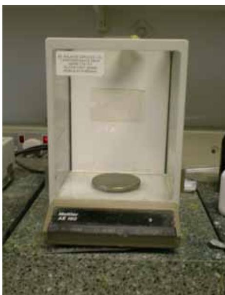
**Figure 3.10** Mettler AE 160 digital balance
