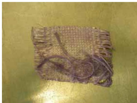
**Figure 3.7** Woven fibreglass
