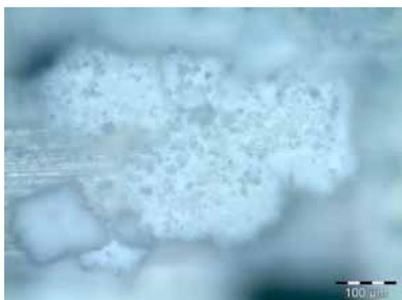
**Figure 3.31** Microscopic image showing the pristine catalyst surface
