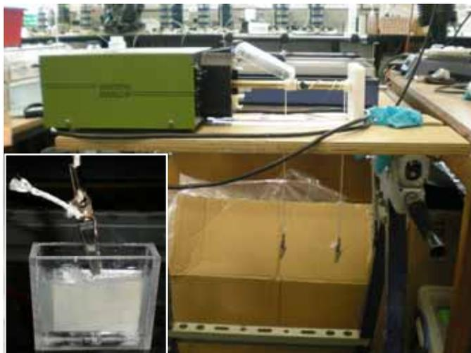
**Figure 3.1** Modified Watson-Marlow 502S peristaltic pump for dip coating, dip coating of a  $12 \text{ cm}^2$  aluminium plate in sol gel (inset)
