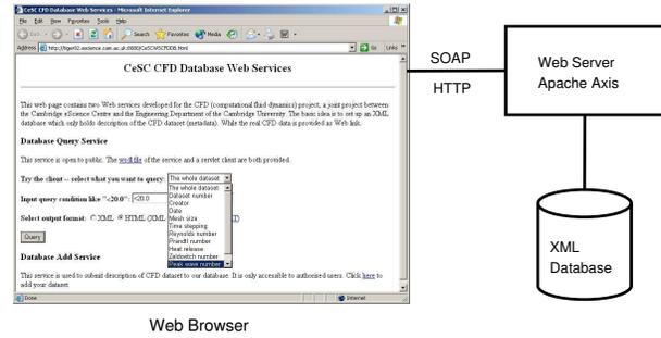
Figure 2. Structure of the CFD query Web service.
