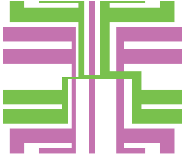
Figure 5.4 Mask design of 90^\circ spin device. Green represents mask for YBCO tracks while pink represents mask for LC(0.3)MO tracks. At the largest YBCO/LC(0.3)MO track junction, the YBCO track width is 8\mu\text{m} .
