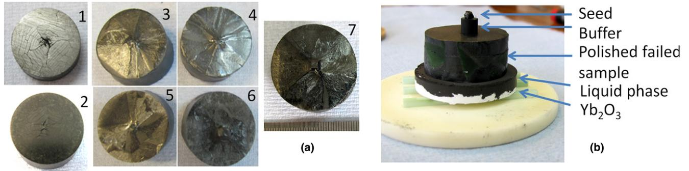
Fig. 1. Procedure for recycling failed Y-Ba-Cu-O samples.
