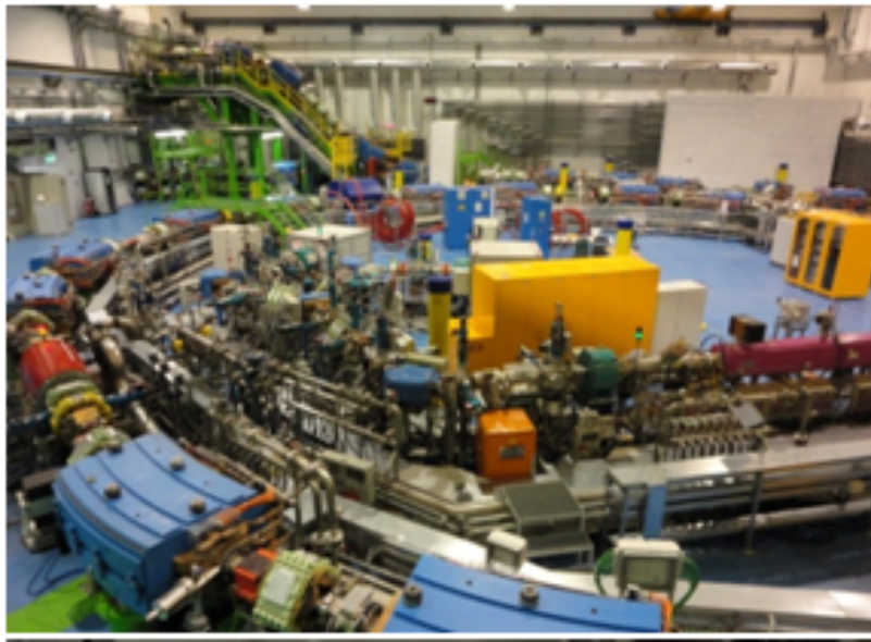
Fig. 1.4 Photograph of the synchrotron at CNAO, Italy used to accelerate high energy protons and carbon ions for patient treatments
