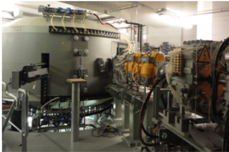
Fig. 1.3 Photograph of the cyclotron at Orsay, which feeds 3 treatment rooms with a high energy of 230MeV
