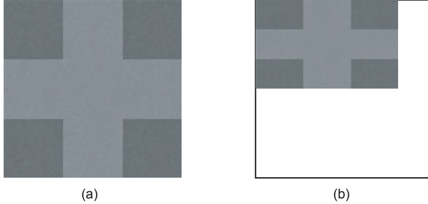
Figure 3.24: (a) A (90 \times 90) image of a cross shape. (b) The same image scaled by a factor of 0.8 horizontally and 0.5 vertically. The pixel intensities in the scaled matrix are determined using bi-cubic interpolation.
