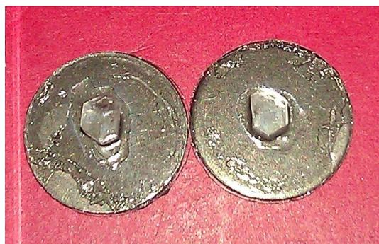
Figure 4.6: Picture of two sections of a large single crystal prepared by cleaving along the length of the crystals. The crystals were glued onto coverslips that were attached to stainless steel discs.
