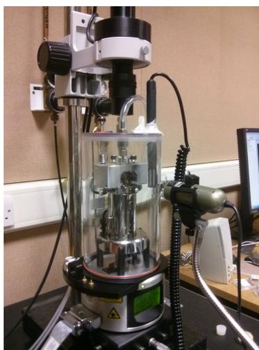
Figure 7.6: Set up for AFM study under controlled humidity level.
