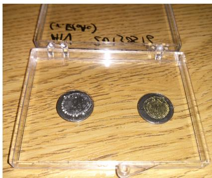
Figure 7.7: Picture of AN crystals before (left) and after (right) exposure to UV light for 1 week.
