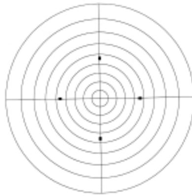
Fig. 6.2 A typical (103) pole figure of *c*-axis oriented YBCO grown on NdGaO<sub>3</sub> substrate.
