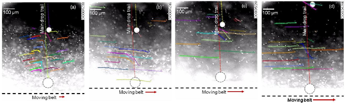
**Figure 5** Disturbance of the gap air flow caused by the passage of a large jetted drop (approximately 80  $\mu\text{m}$  in diameter, travelling at  $\sim 3.3$  m/s) with substrate speeds of a) 0.5 m/s, b) 1.0 m/s, c) 1.5 m/s, and d) 2 m/s.
