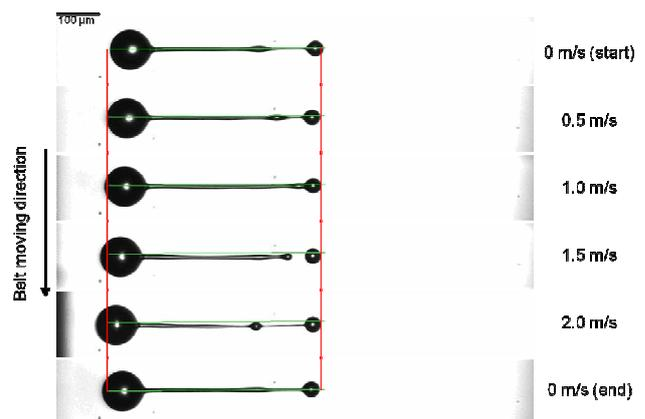
**Figure 3** Jetted ethylene glycol drops, ligaments, and satellites moving from right to left across the print gap at belt (substrate) speeds from 0 to 2 m/s.
