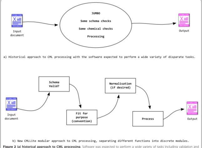
**Figure 2 (a) historical approach to CML processing**. Software was expected to perform a wide variety of tasks including validation and transformations (processing). (b) the CMLLite approach: each module performs only one task *i.e.* validation, normalisation or transformation (processing). This makes each of the modules more straightforward to understand and produces cleaner code.
