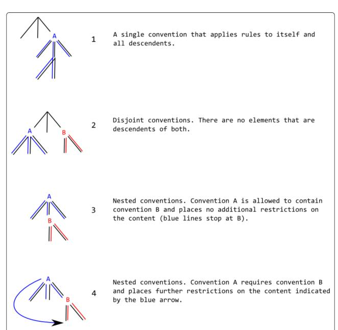
**Figure 7 Documents with multiple conventions**. The black lines represents the XML tree (DOM) and are shadowed by constraints imposed by conventions A (blue) and B (red).
