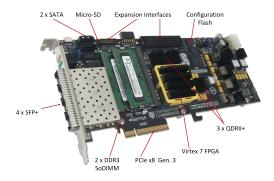
Figure 1: NetFPGA SUME Board
