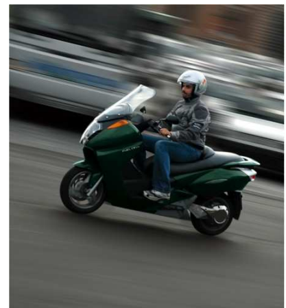
Figure 20.44. Vectrix: 2.75 kWh per 100 km . Photo from www.vectrix.com .
