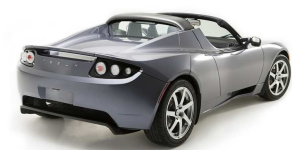
Figure 20.22. Tesla Roadster: 15 kWh per 100 km . www.teslamotors.com .
