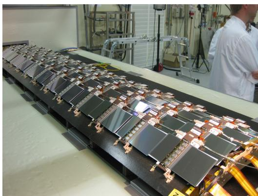
(c) The completed sector mounted with 48 barrel modules.
