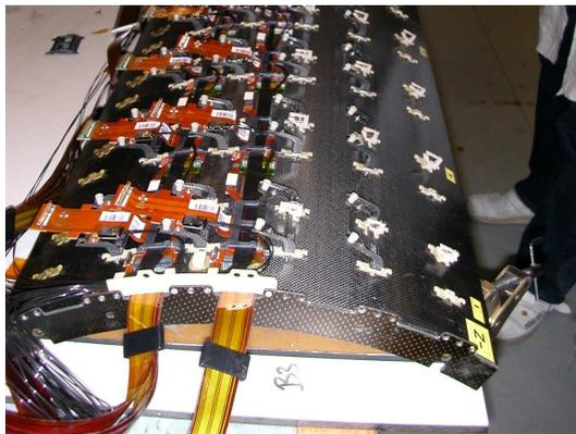
(a) Two harnesses mounted on the sector. The orange low mass tapes and black readout fibres are clearly visible.
