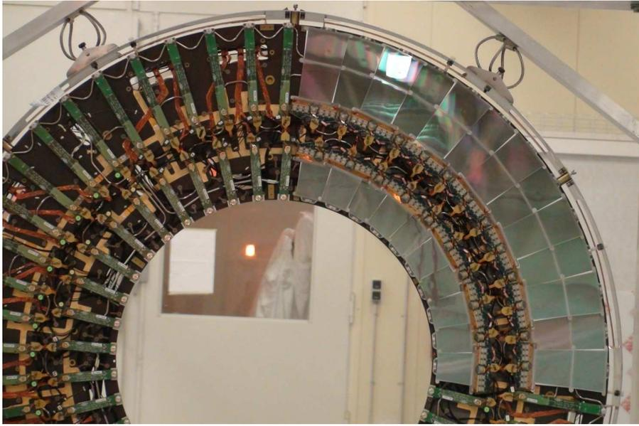
**Figure 4.3:** The spare end-cap disk showing outer and inner modules, viewed from  $z = 0$  as indicated in figure 4.1. The middle modules are mounted on the reverse of the disk and are not visible here.
