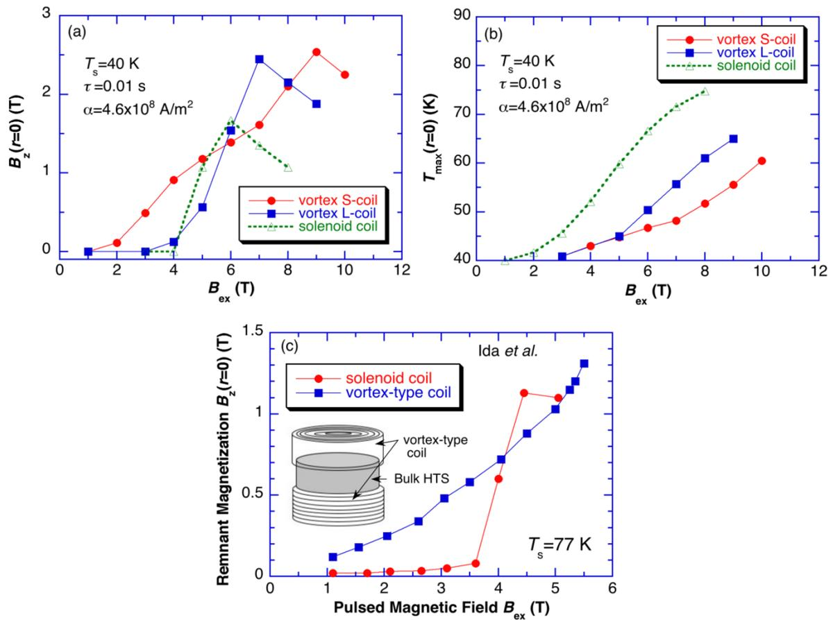
Figure 10. (a) Trapped field  $B_z(r=0)$  and (b) maximum temperature  $T_{max}(r=0)$  at the centre of the bulk surface as a function of applied field  $B_{ex}$  using the three coils (vortex S-coil, vortex L-coil and solenoid coil) shown in Figure 9 [128]. (c) Reported experimental results by *Ida et al.* in [157].
