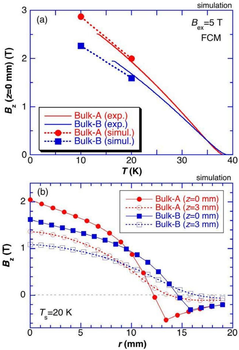
Figure 7. (a) Simulation results for the trapped field  $B_z$  ( $z = 0$  mm) at 10 and 20 K for each MgB<sub>2</sub> bulk. The solid lines show the experimental results. (b) Cross-sections of the trapped field profiles at 20 K for each bulk at  $z = 0$  (bulk surface) and 3 mm [127].
