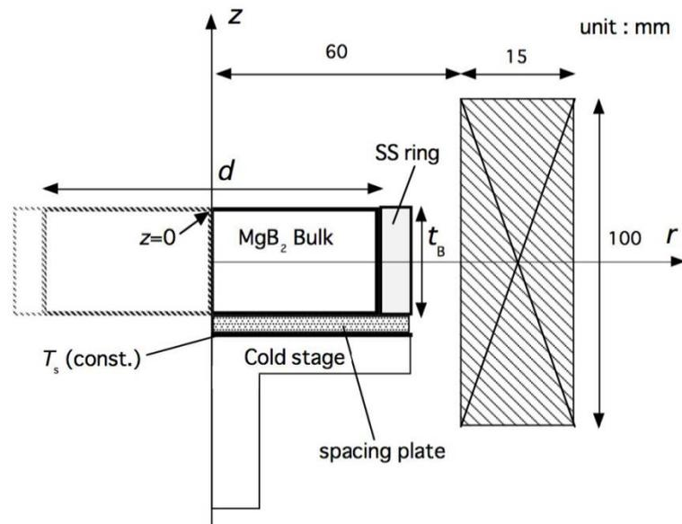
Figure 5. Schematic view of the experimental setup and the basis for the numerical model of bulk  $MgB_2$  superconducting discs magnetized by FC presented in [127].
