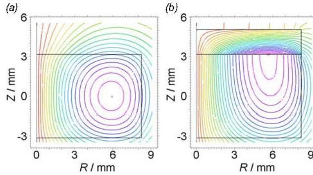
Figure 17. (a) Contour lines of the vector potential  $\mathbf{A}$  in the fully magnetized remanent state for the superconductor without any ferromagnetic alloy addition in [97]. The results are obtained by solving Campbell's equation [63,82]. (b) The same contour lines for the hybrid ferromagnet-superconductor structure C1 shown in Figure 16.
