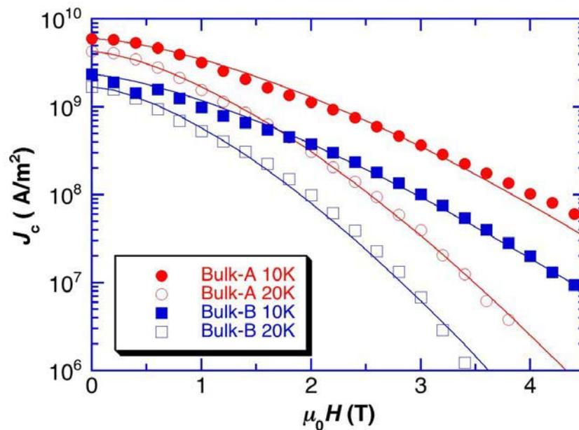
Figure 6. Estimated  $J_c(B)$  characteristics for both  $MgB_2$  bulks in [127] at 10 K and 20 K. The solid lines show the fitting curves used in the simulation.
