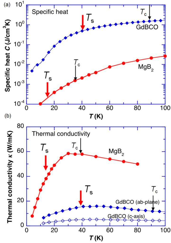
Figure 3. Comparison for MgB<sub>2</sub> and (RE)BCO bulk superconductors of (a) Specific heat and (b) Thermal conductivity.
