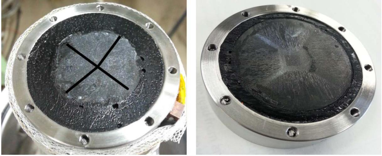
Figure 2. YBCO (left) and GdBCO (right) bulk superconductor samples. The growth sector boundaries (GSBs) are shown for each sample [82].
