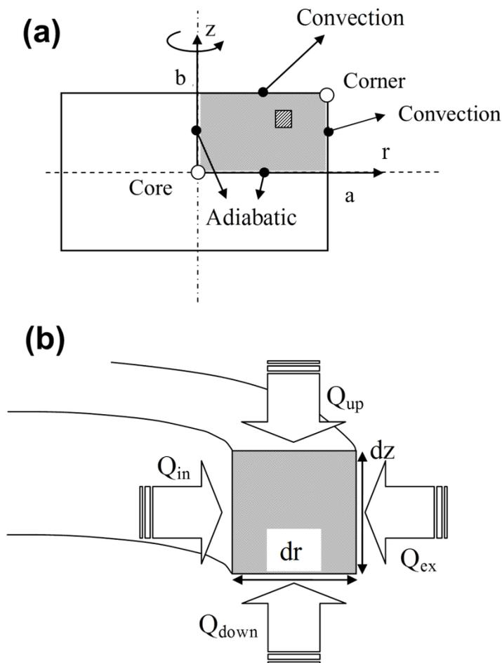
Figure 12. (a) Cross-section of the superconducting disc modelled in [176] showing the thermal boundary conditions. The lateral ( $r = a$ ) and top ( $z = b$ ) surfaces exchange heat with the cryogenic fluid by convection. The central plane ( $z = 0$ ) and the axis ( $r = 0$ ) are adiabatic. (b) Cross-section of a ring element of width  $\Delta r$  and thickness  $\Delta z$ . The heat flux directions,  $Q_{up}$ ,  $Q_{down}$ ,  $Q_{in}$  and  $Q_{ex}$ , are indicated by the arrows.
