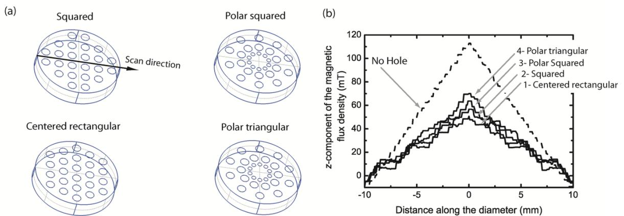
Figure 15. (a) The four lattices of drilled holes analysed numerically in [36]. (b) Trapped field profiles along the bulk diameter calculated by the model, with a sweep rate of 10 mT/s and  $n = 25$ , including a reference bulk superconductor without holes.
