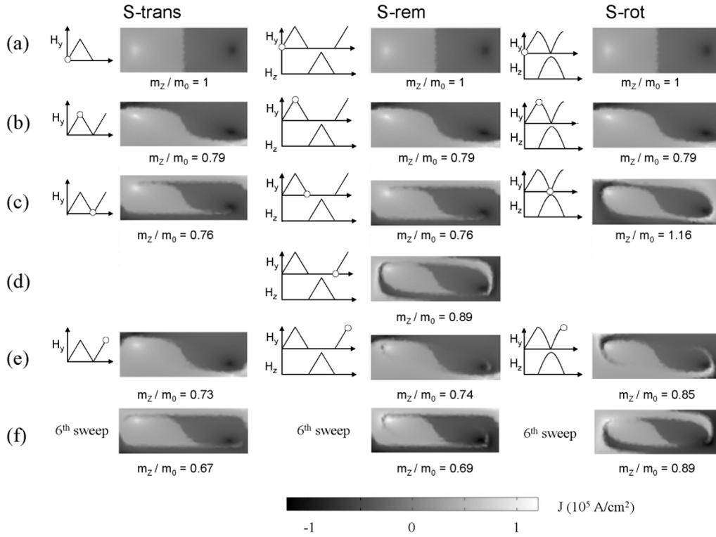
Figure 11. Modelled data of the complex current density distributions  $J_x(y,z)$  within the cross-section of the bulk sample at selected times during each of three cycles of an applied magnetic field of magnitude  $H_{\max} = 0.5H_p$ . The magnetic moment normalised to the initial value,  $m_z/m_0$ , is also given below each current distribution. More details on the configuration of the applied fields can be found in [162].
