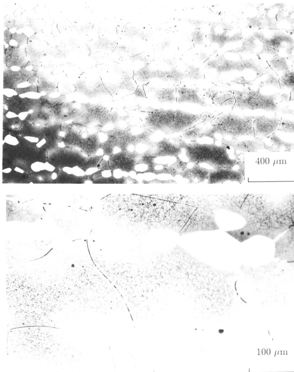
Figure 5.19. Light micrographs showing the microstructure of duplex rolled metal IC381 solution treated at 1300 °C for 26 hours and then quenched into water. The light phase is austenite and the dark one is ferrite. TEM observations (Figure 5.22) show that the fine particles inside the ferrite grains are austenite formed during quenching. The measured volume fraction of austenite (excluding fine particles) is about 0.19.
