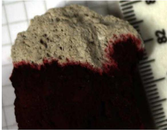
**Figure 5.3:** Photograph showing the saturation of a pumice fragment with red food dye. At the edge of the wetted portion of the pumice, there is a region of partial saturation, illustrated by the colour variation in this region.
