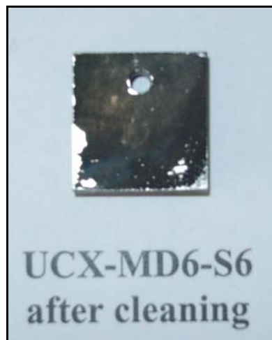
(b) Alloy condition after 500h
