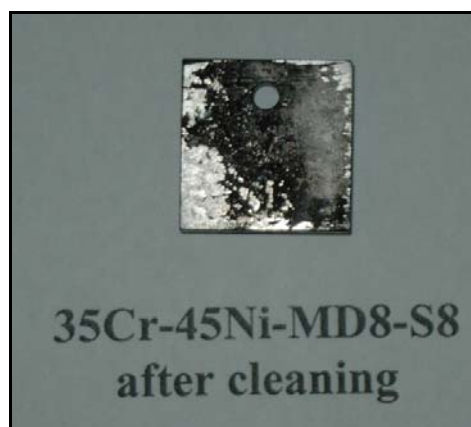
(c) Alloy condition after 1000h
