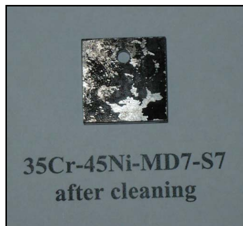
(c) Alloy condition after 1000h
