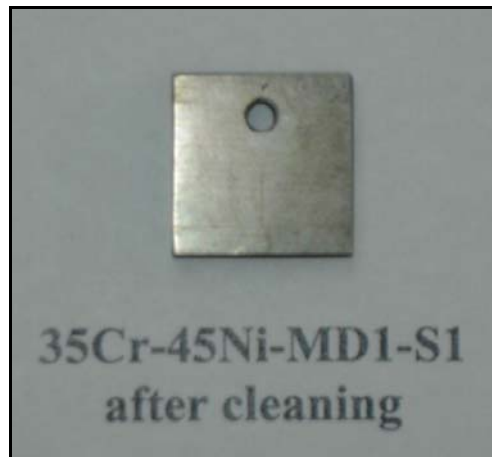
(a) Alloy condition after 100h
