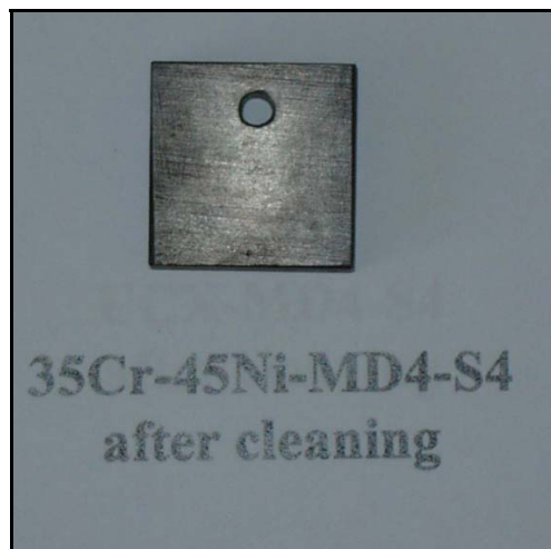
(b) Alloy condition after 500h
