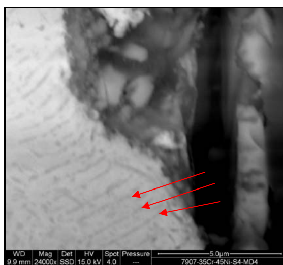
Figure 6.33 Carburisation (in form of parallel strips indicated by arrows) was observed at the substrate (under the pit).
