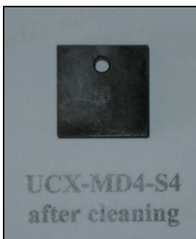
(b) Alloy condition after 500h
