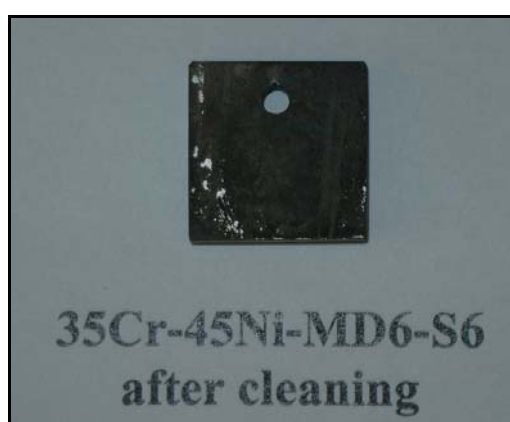
(b) Alloy condition after 500h
