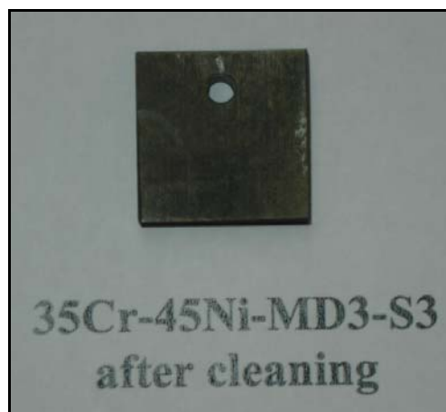
(a) Alloy condition after 100h
