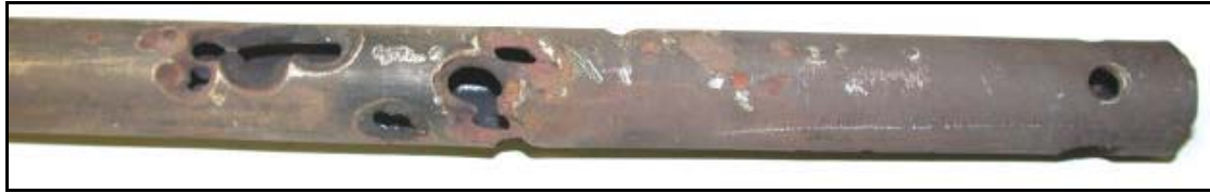
Figure 1.3 Metal dusting in alloy RA330 tube used in heat-treating environments at about 930°C [7].
