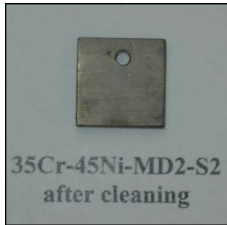
(a) Alloy condition after 100h
