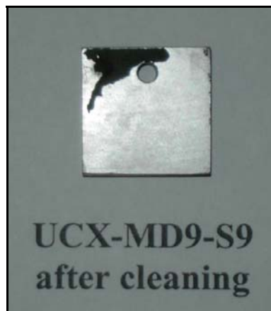
(c) Alloy condition after 1000h
