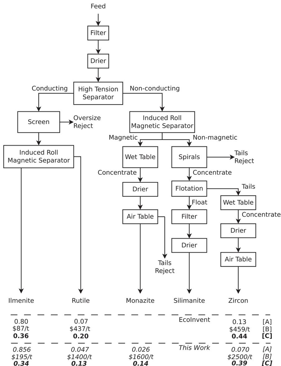
**Fig. 3.** Flow sheet for the production of monazite, adapted from Ref. [25]. [A] denotes the relative abundance of the mineral; [B] denotes the economic value of the mineral; and [C] denotes the normalised weight from the product of [A] and [B]. Original data used for the Ecolnvent weighting are presented in normal text with the weightings used (derived from 2011 US) values in Ref. [26] in italic text.
