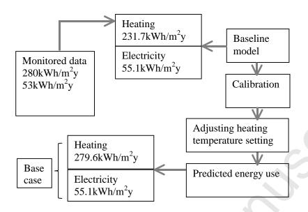
Fig.3. Structure of the validation and calibration process
