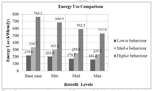
**Fig.6.** Energy use comparison among different retrofit levels with three behavioural scenarios
