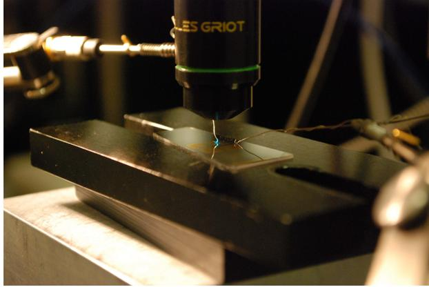
**Figure 5.2:** Custom experimental photovoltaic set-up allowing microscopic control of prober tip location and simultaneous electrical and optical characterisation.
