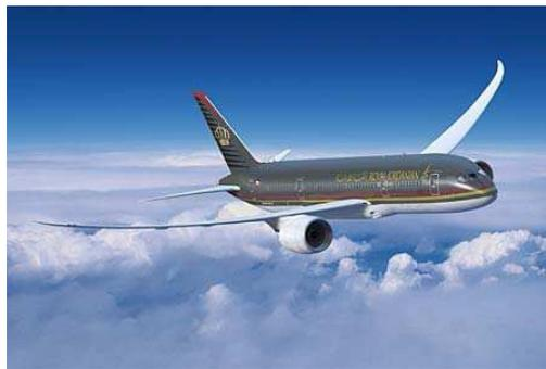
Figure 1.1: Conventional aircraft layout — the Boeing 787 Dreamliner.
