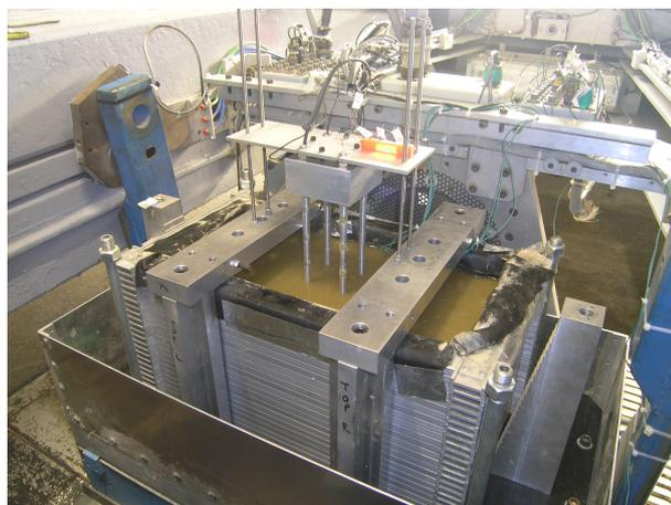
Figure 3.18: Installation of heavily instrumented pile group at 1g
