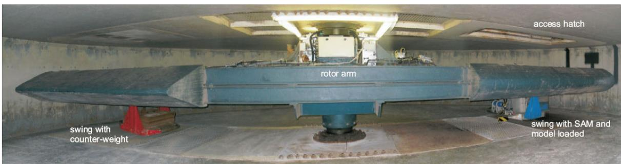
Figure 3.1: The Turner beam centrifuge. Photo: Steve Chandler
